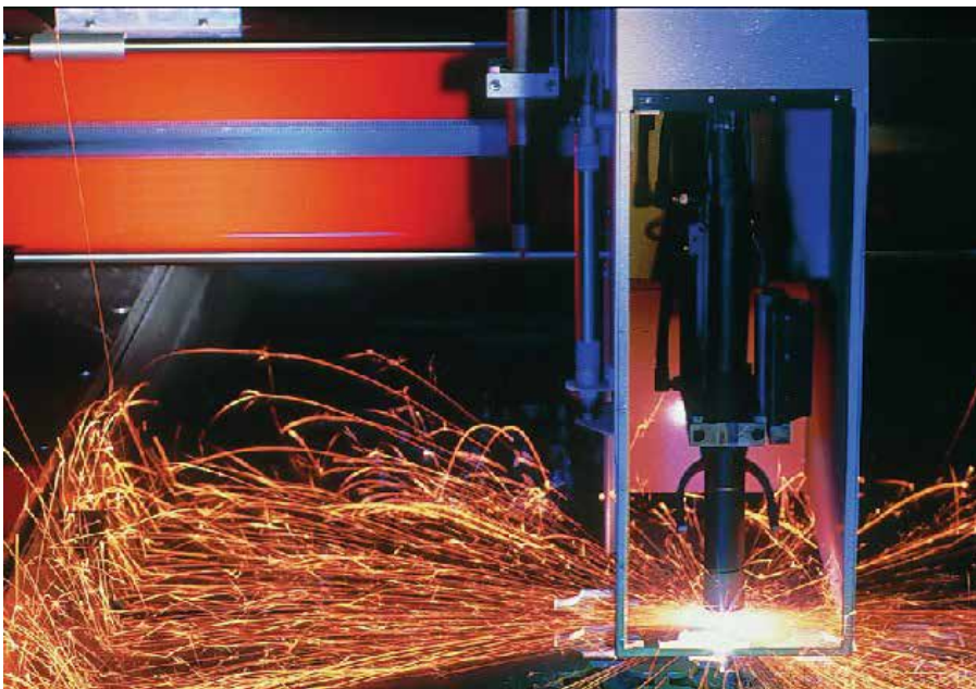
Fig. 2. Plasma cutting process for metal plates
