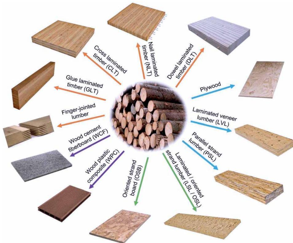
**Figure 1.** Major types of engineered wood products and their abbreviations (source: images obtained from archiproducts.com, canac.ca, diy.com, globalsources.com, leben.co.in, nrcan.gc.ca, and structurecraft.com).
