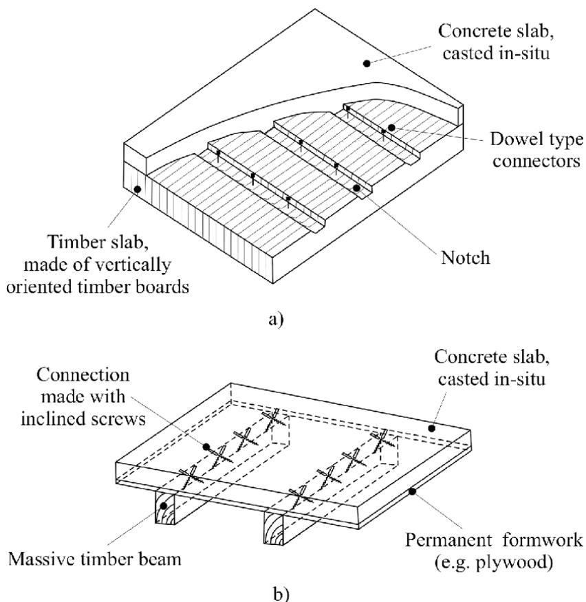
**Figure 2.** Examples of slab type and beam type of TCC floor systems. (a) An example of slab type of TCC floors. (b) An example of beam type of TCC floors.
