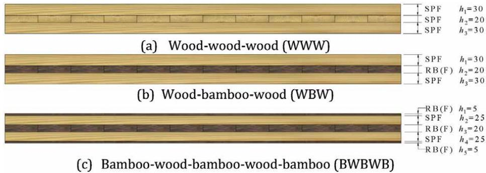
**Figure 14.** Configuration of bending specimen of CLT and CLTB (unit: mm). (a) Wood-wood-wood (WWW), (b) wood-bamboo-wood (WBW), (c) bamboo-wood-bamboo-wood-bamboo (BWBWB) (adapted from dong, [46]).
