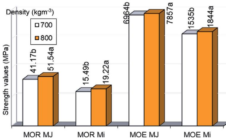
**Figure 4.** Effect of board density on bending properties.
