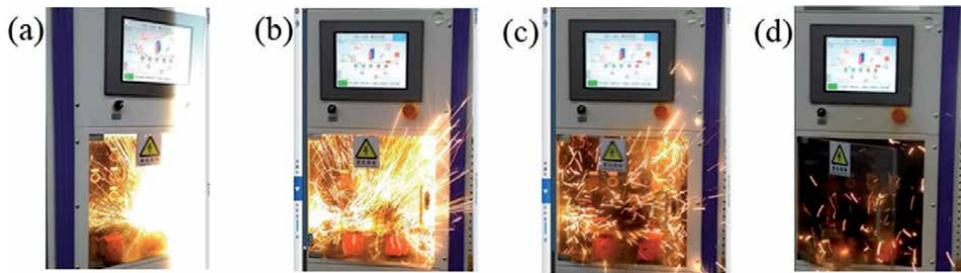
**Figure 8.** The process for the timber being struck by lightning. (a) A strong white light instantly appeared and then disappeared quickly. (b) Then a large amount of dazzling scattered sparks near the surface of the timber. After that, the sparks slowly weakened and its number slowly decreased in (c) and (d). Each picture was separated by 10-20 milliseconds.
