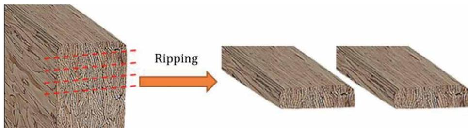
**Figure 12.** Boards ripped from PSL (source: photos adopted from Gouldsdesigninc.com [52]).
