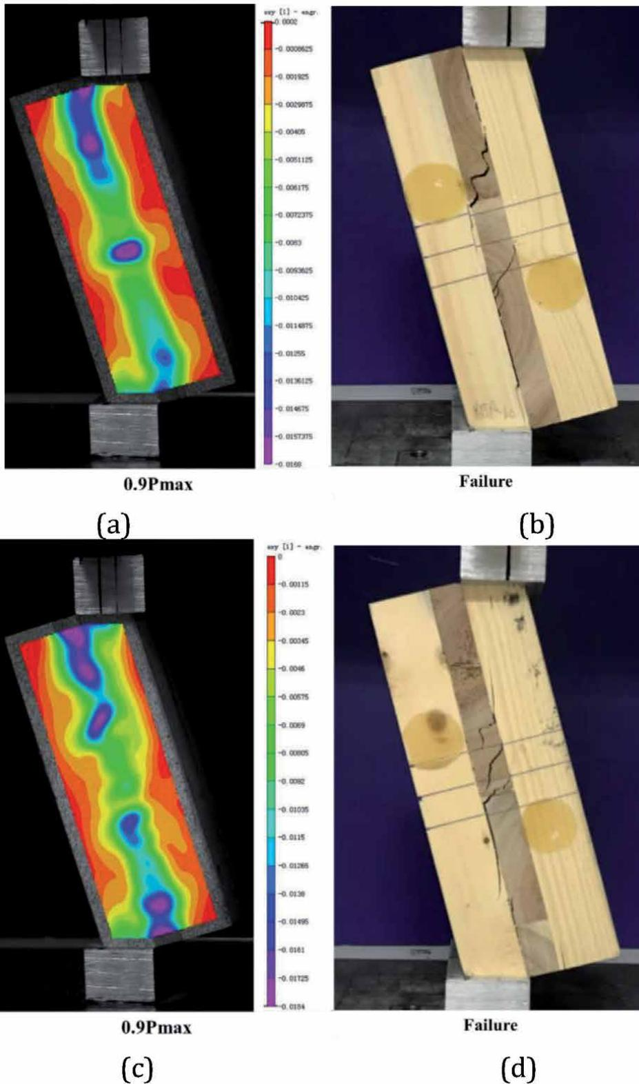
**Figure 11.** Strain distribution and failure of eucalyptus CLT specimens under rolling shear: (a) and (b) width-thickness ratio ( $\gamma$ ) = 4, and (c) and (d)  $\gamma$  = 6 (adapted from Gui et al. [26]).
