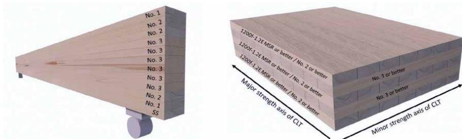
**Figure 11.** Design of GLT (left) and CLT (right) [9].
