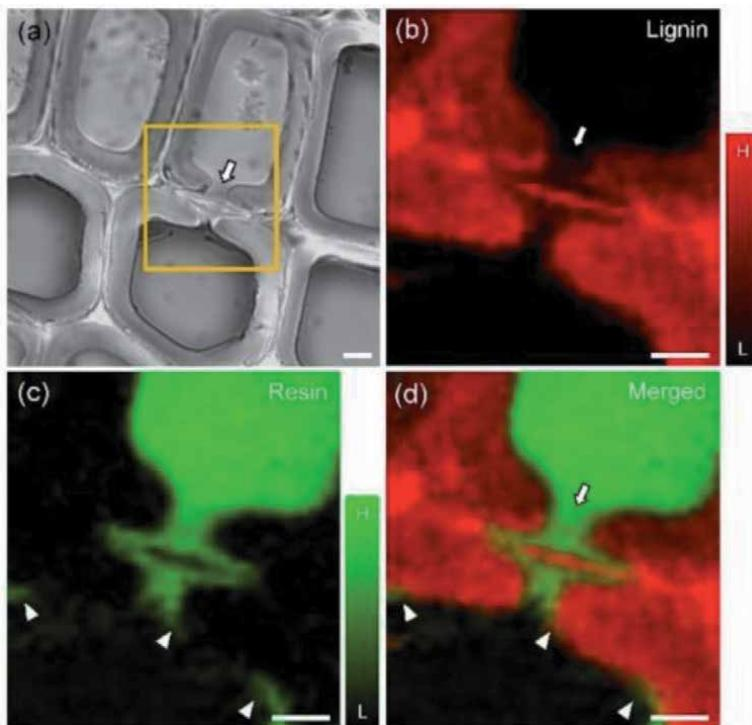
**Figure 29.** Raman mapping on cross section of coated samples of Japanese cedar (a) Raman image (b) lignin, (c) alkyl resin and (d) merged information adrenal glands [65].
