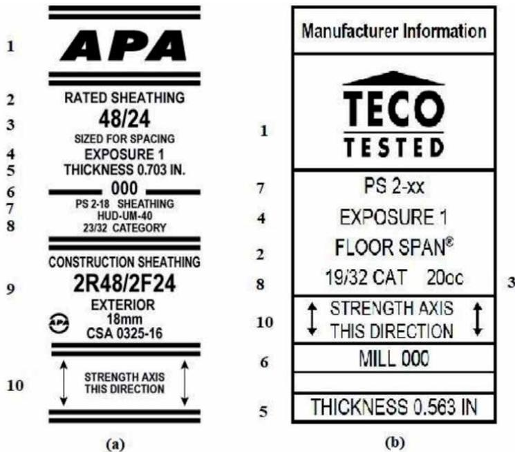
**Figure 4.** Typical grade stamps for OSB: (a) APA grade stamp; and (b) TECO grade stamp. (1. Third-party inspection agency; 2. Panel grade; 3. Span rating; 4. Bond classification; 5. Thickness; 6. Mill number; 7. Product standards; 8. Performance category; 9. Canadian construction sheathing standard; 10. Panel face orientation indicator. Source: Pictures obtained from APA at <https://www.apawood.org/apa-trademark> and TECO at <https://www.pfsteco.com>).
