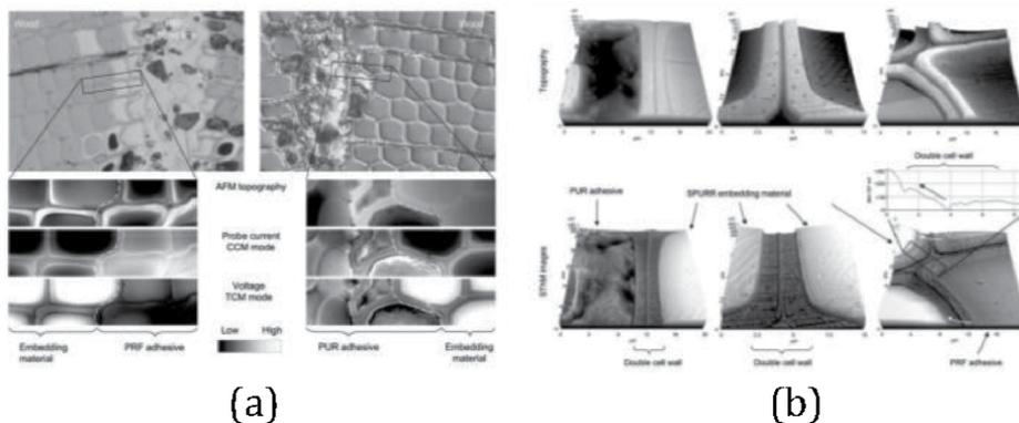
**Figure 17.** (a) Images of adhesive bond in spruce samples using (top): Light microscopy and (bottom): SThM mapping the topography, probe current and voltage and (b) differences in topography for SPURR epoxy resin (Centre) and in contact with PUR adhesive (left) and PRF adhesive (right).
