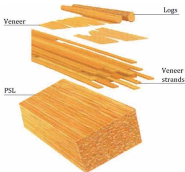
**Figure 11.** Orientation of veneer strands in PSL (source: photos obtained from WorldPress.com [50]).
