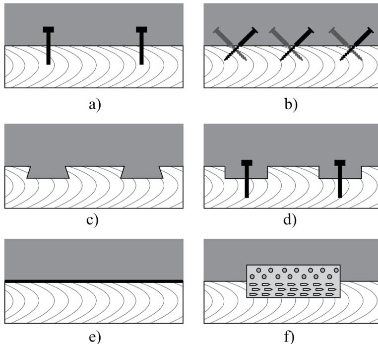
**Figure 3.** Connection types. (a) Connection with dowels. (b) Connection with inclined screws at  $45^\circ$  in two rows. (c) Notched connection with inclined sides. (d) Notched connection with vertical sides and dowels. (e) Glued connection. (f) Connection with nailplates.
