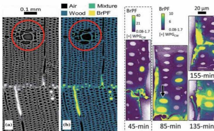
**Figure 21.** Left- X-ray computed tomography (XCT) and right- X-ray fluorescence microscopy (XFM) images of glue line [58].
