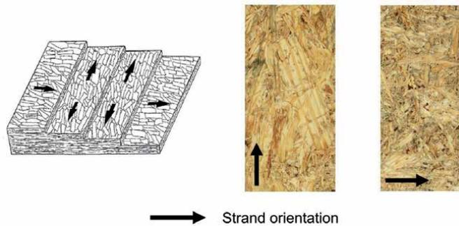
**Figure 2.** Strand orientation of OSB panels: Schematic (left) (source: Picture obtained from FAPC) [18]; large-size strands in the surface layer (center) and small-size strands in the core layer (right).
