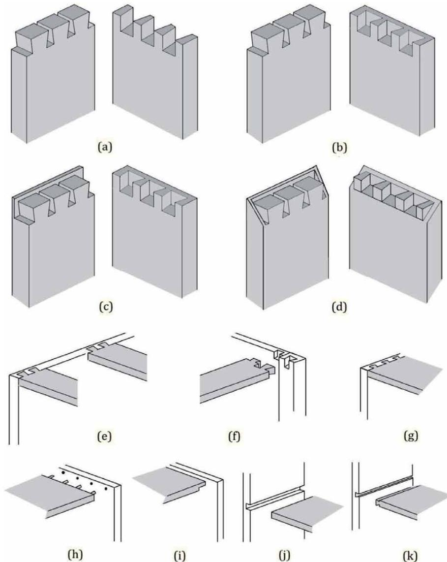
**Figure 11.** Examples of dovetail joints in wooden furniture design: (a) through dovetail, (b) lapped dovetail, (c) double lapped dovetail, (d) secret mitred dovetail. Joints used in carcasses: (e) cross rails dovetailed into solid side, (f) cross rails dovetailed into framed side, (g) top dovetailed to side, (h) top dowelled to side, (i) top rebated, (j) housing, (k) tapered dovetail housing (drawn by Emre ILGIN).
