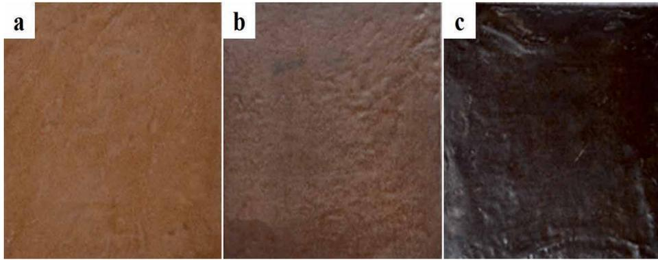
**Figure 14.** The HEPE-based WPC with RSS modified by various superheated vapor temperatures: a. control, b. 200°C, c. 220°C [37].
