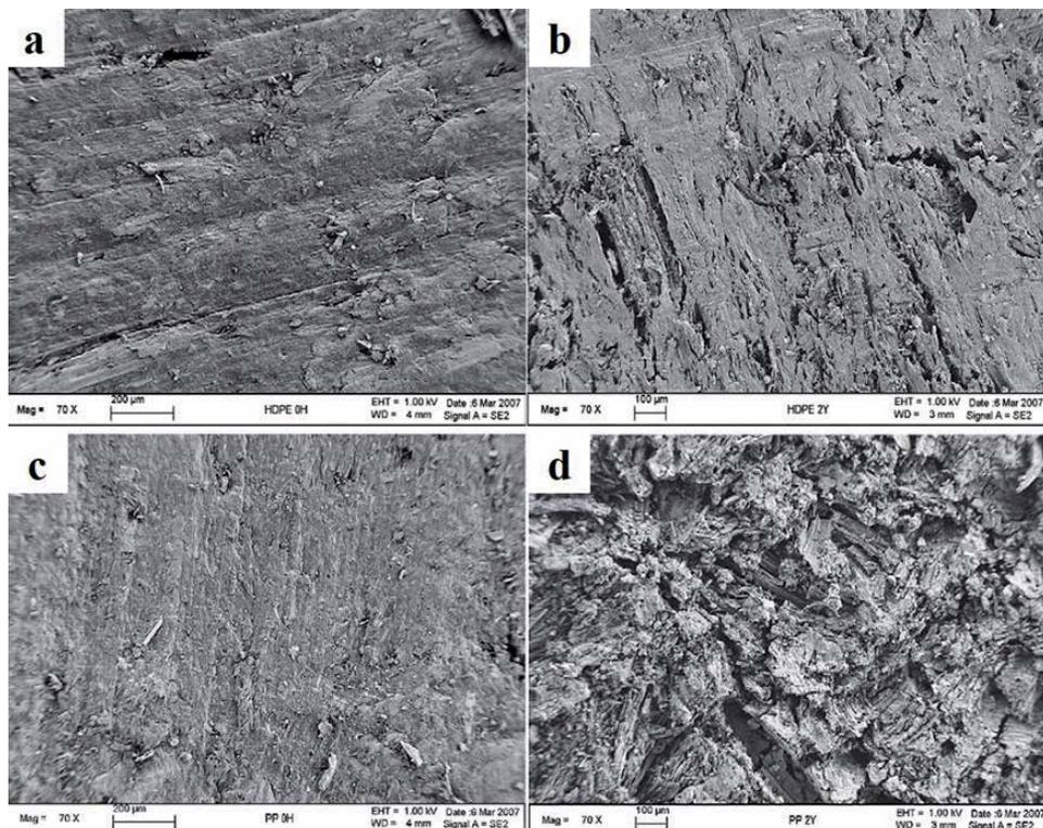
**Figure 11.** Scanning electron micrographs of various WPCs before and after weathering: a, c. HDPE-based and PP-based WPC that was unweathered, respectively; b, d. HDPE-based and PP-based WPC that 2-yr exterior-weathered, respectively [23].
