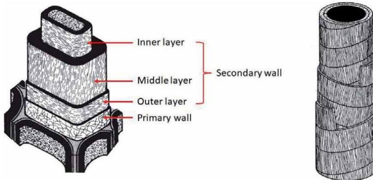
**Figure 14.** The hierarchical structure of a mature cell wall (left) (adapted from [21]) and a cylindrical LVL (right) (adapted from [22]).
