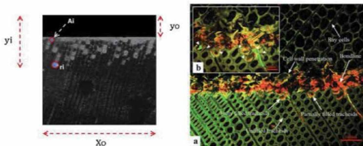
**Figure 2.** (Left) Imaging of effective penetration (EP) and maximum penetration (MP) of gross penetration of into structure [8] and (right) penetration of urea formaldehyde (UF) into wood cell walls shown in green colour [9].
