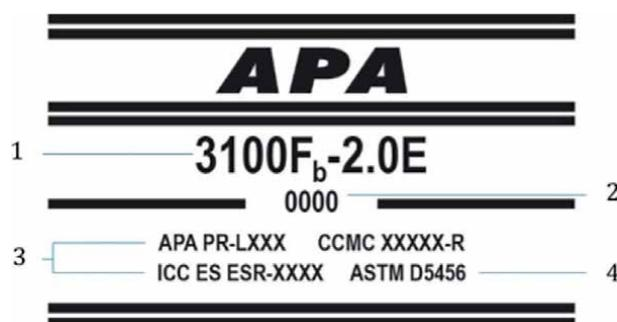
**Figure 9.** LVL stamp: 1 – qualified LVL grade (usually represented by design values; 2 – APA mill number; 3 – product evaluation reports; 4 – standard specification for structural composite lumber (source: photo obtained from APA – the Engineered Wood Association).
