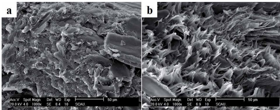
**Figure 15.** Micro-morphology of the HDPE/RSS composites with unmodified and modified RSS by superheated vapor: a. unmodified, b. modified [37].
