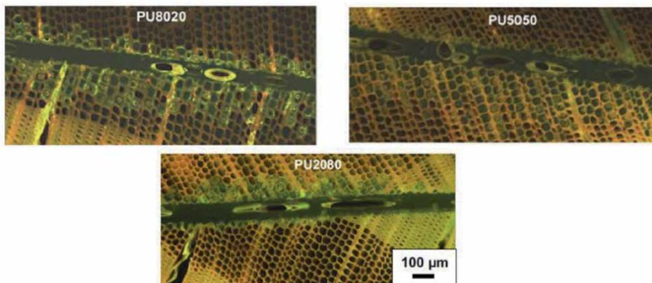
**Figure 8.** Florescence microscopy imaging of PUR bond line and penetration development for top: PU8020 with 53.5%, middle: PU5050 with 65.4% and bottom: PU2080 with 72.5% hard phase mass [35].
