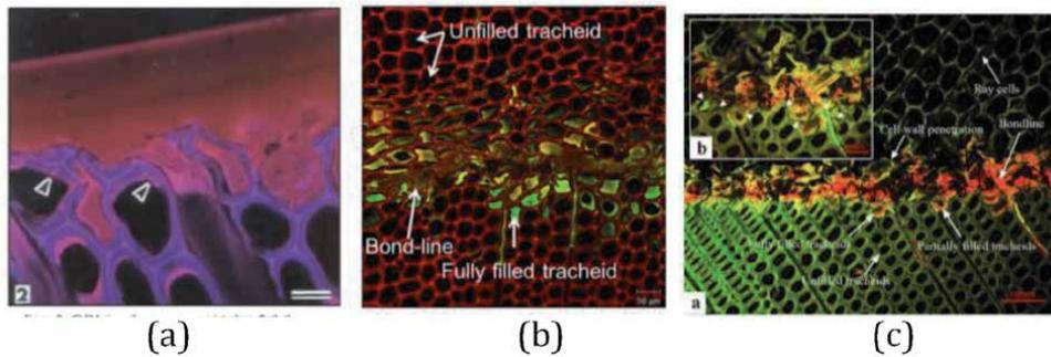
**Figure 26.** CLSM used in (a) imaging coating surface and penetration of coating material into the wood structure (bar = 20  $\mu\text{m}$ ) [61], (b) urea formaldehyde (UF) resin penetration into wood structure [62] and (c) UF adhesive imaging showing wood structure and resin penetration [9].
