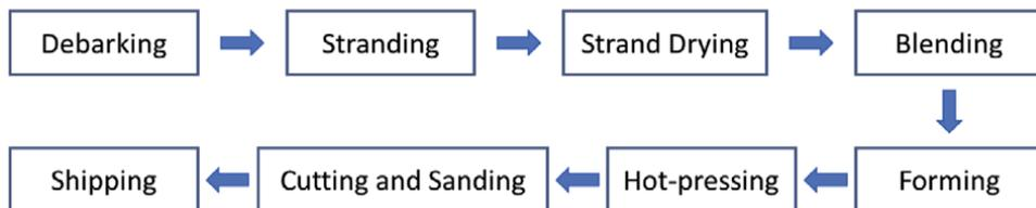
**Figure 3.** The key manufacturing processes of OSB.
