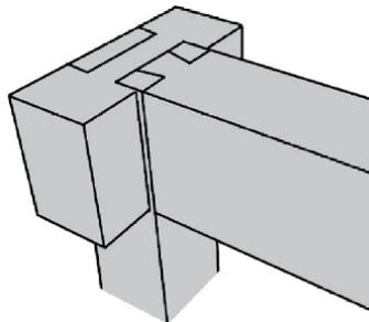
**Figure 7.** The dovetail joint for the test specimen (drawn by Emre ILGIN).
