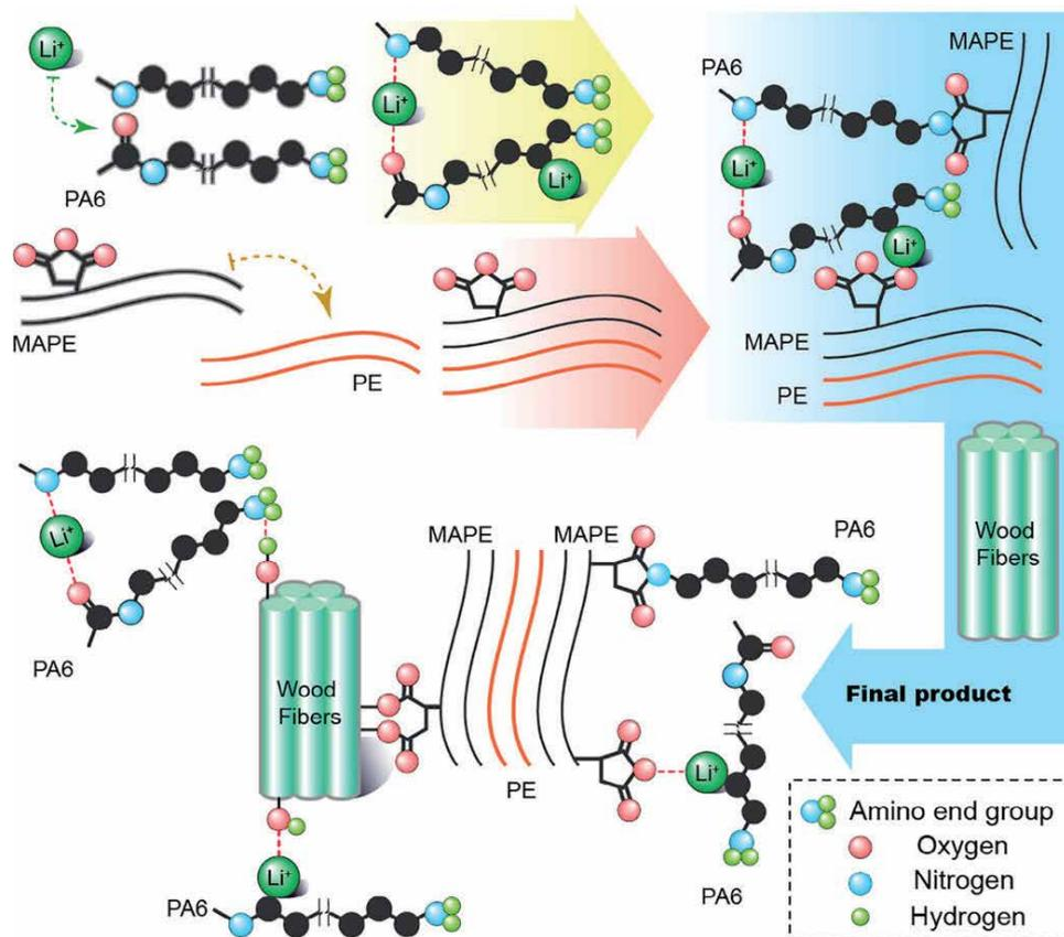
**Figure 12.** Reaction mechanism diagram of  $\text{LiCl}$  and MA-g-PE in PE-based WPC [32].
