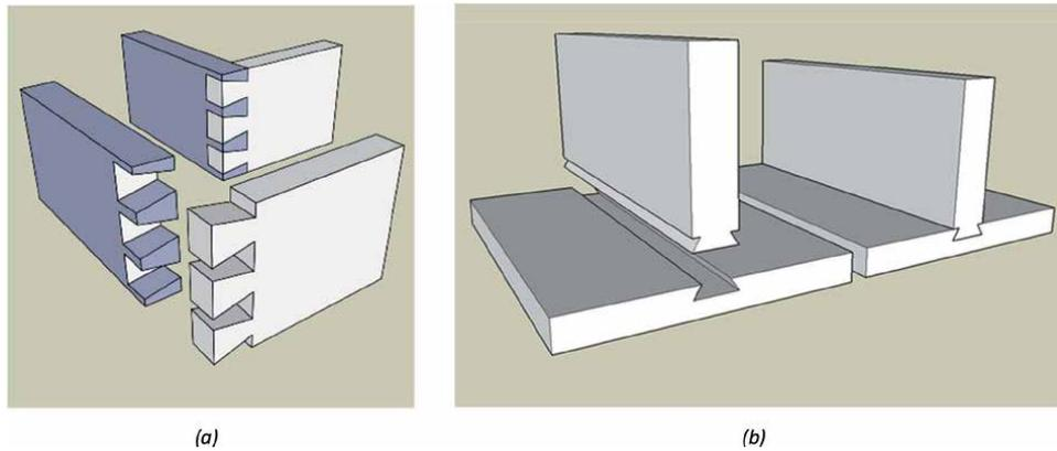
**Figure 4.** *Dovetail joint as one of the oldest joining techniques in furniture design: (a) a through dovetail joint; (b) a sliding dovetail joint (sources: Wikipedia—[https://en.wikipedia.org/wiki/Dovetail\\_joint](https://en.wikipedia.org/wiki/Dovetail_joint)).*
