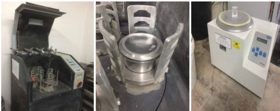
Figure 1. Laboratory grinder and air-jet sieve for collecting ground PC clinker.
