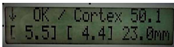
Figure 14. The result of the drilling process; new drill bit 2.8 mm.
