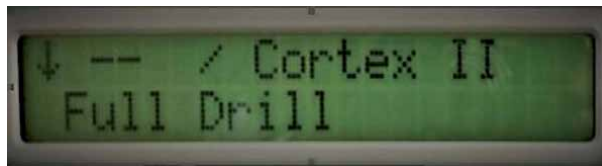
Figure 4. “Cortex II full drill” mode - bicortical drilling and automatic stop after second cortex end registration.
