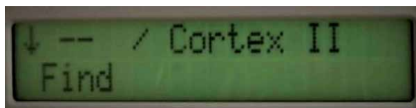
Figure 5. “Cortex II find” mode - drill bit detection the far cortex wall from inside and stop automatically.
