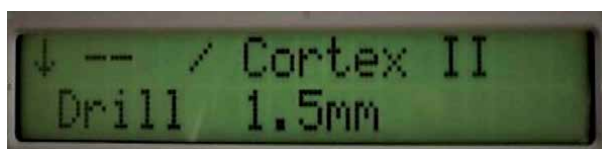
Figure 6. “Cortex II drill” mode - drilling through the near (first) cortex and partially the far (second) one, making a hole with a 1.5 depth in [mm].
