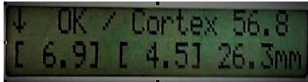
Figure 15. The result of the drilling process; hole-used 35 times drill bit 2.8 mm.
