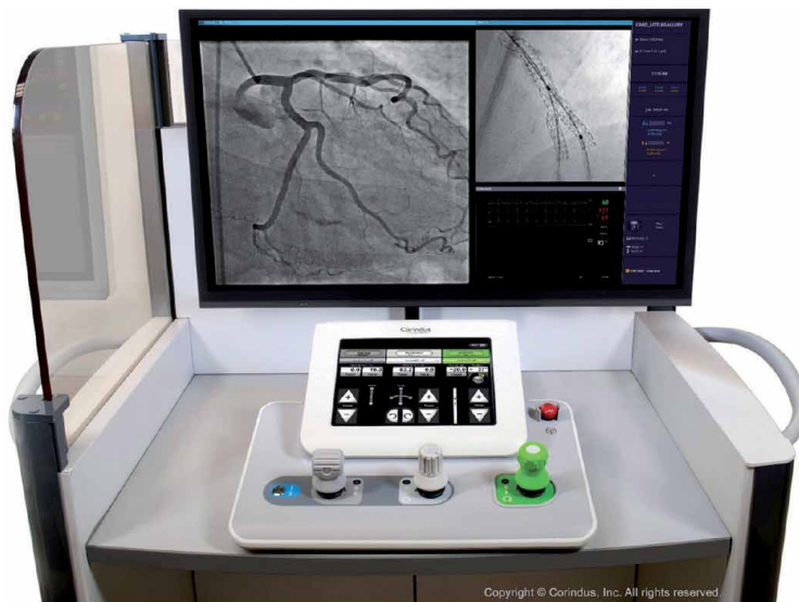
Figure 1. Robotic console workstation with radiation shielding. The monitors show live fluoroscopy images and patient vitals (© Corindus Inc., used with permission) [5].
