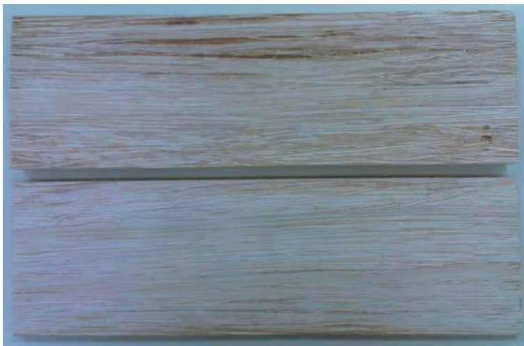
Figure 20. Composite board from compressed oil palm fronds were trimmed.
