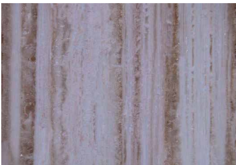
Figure 25. High-performance micrograph of the urea-formaldehyde composite board from compressed oil palm fronds at the longitudinal sectional view (2× magnification).
