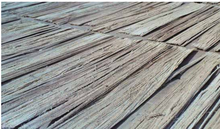
Figure 18. Compressed oil palm fronds under sun-drying.
