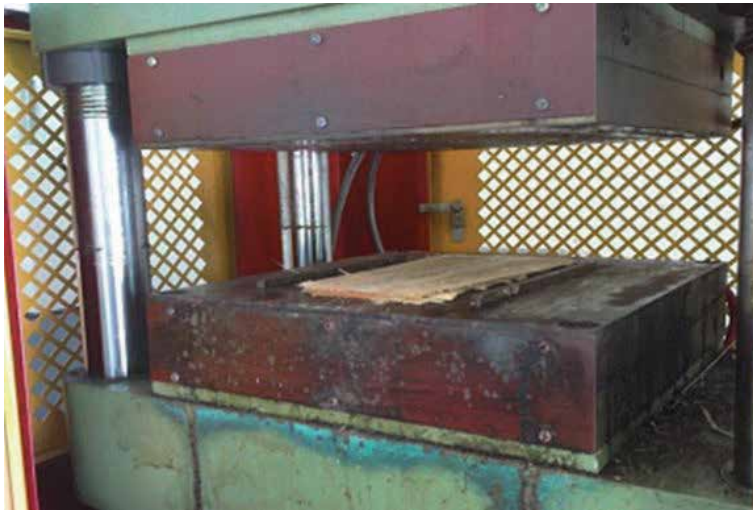
Figure 19. Layers of palm oil fronds being compressed using a hotpress machine.
