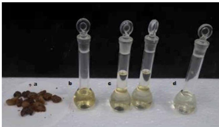
Figure 6. Products obtained from the biodiesel processing steps. Caption: a: gongo sludge; b: gongo oil in natura; c: esterified gongo oil and d: gongo biodiesel [20].
