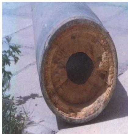
**Figure 1.** *Scaling through  $\text{CaCO}_3$  precipitation in drinking water pipes.*
