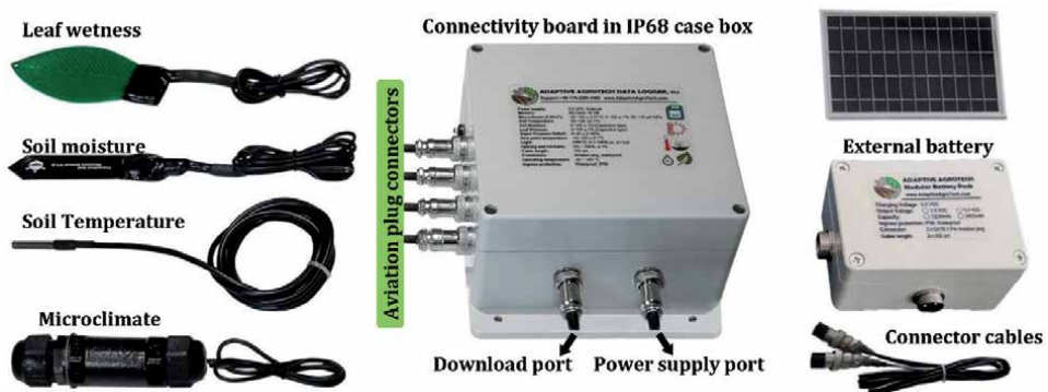
Figure 8. A hybrid data acquisition system with modular solar charged external battery, plug-and-sense probes, 32GB onboard, and multiple communication interfaces for data transfer including serial port, WiFi, and LoRa 868Mhz. Image by courtesy of Adaptive AgroTech.
