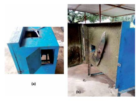
Figure 5. Partial view of the chopping machine brand ITARA-M 9186/BI. (a) Outside view and (b) Chainsaw part.
