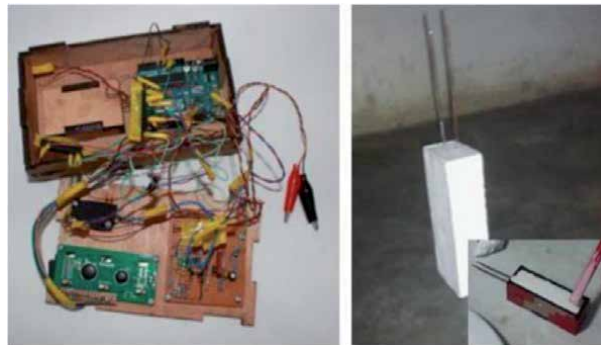
Figure 11. Soil moisture sensor and Arduino reader with LCD display [33].
