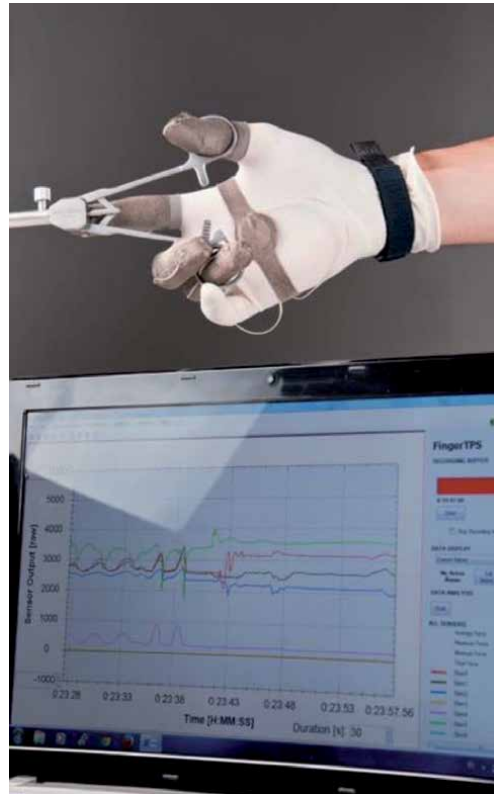
Figure 5. Use of the FingerTPS™ system during the handling of laparoscopic instruments with a ring handle. (Source: [3]).
