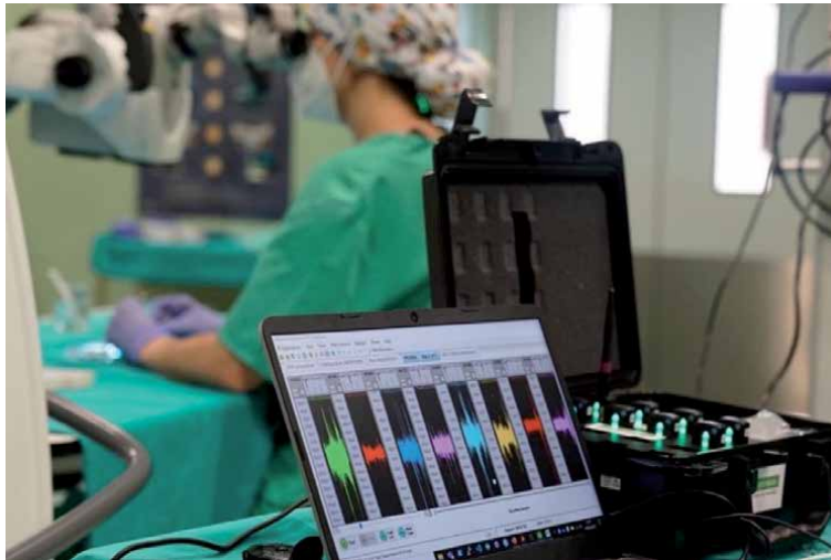
Figure 2. Use of the Delsys Trigno™ EMG wireless system as a tool for recording sEMG and motion data to assess the surgeon's posture and workload in microsurgery.
