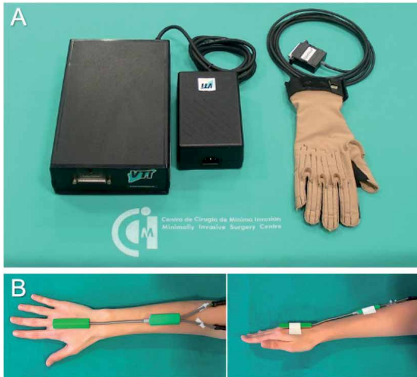
Figure 4. Use of the CyberGlove™ device (A) and an electrogoniometer (B) for recording the surgeon's hand posture during laparoscopic practice. (Source: [17]).
