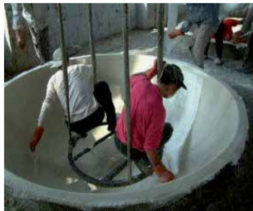
Figure 5. Hand fabrication of composite material digester model in China. Image courtesy: Shikun Cheng.
