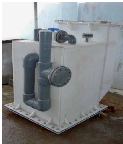
Figure 7. Compact, high-rate digester for kitchen organic waste disposal. Image courtesy: Shikun Cheng.
