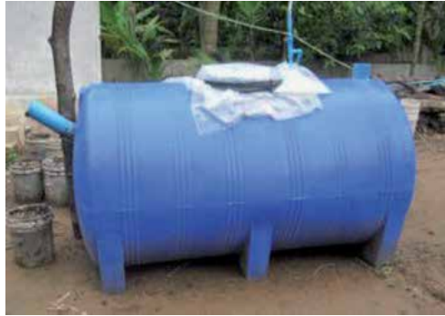
Figure 6. Commercial water tank (composite material digester) in Cambodia. Image courtesy: Shikun Cheng.
