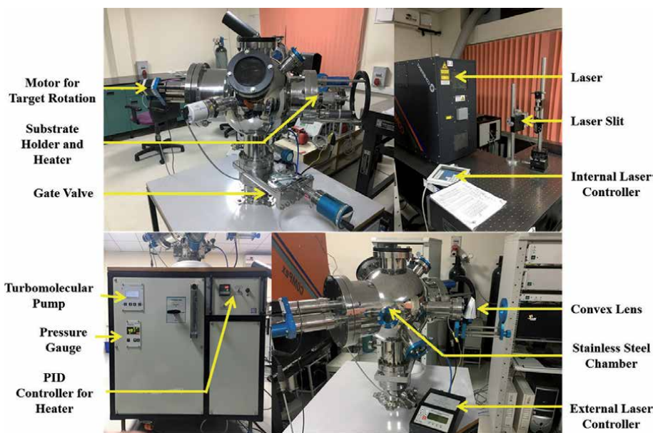
Figure 3. PLD setup in Materials Research Centre, Indian Institute of Science, Bangalore, India.
