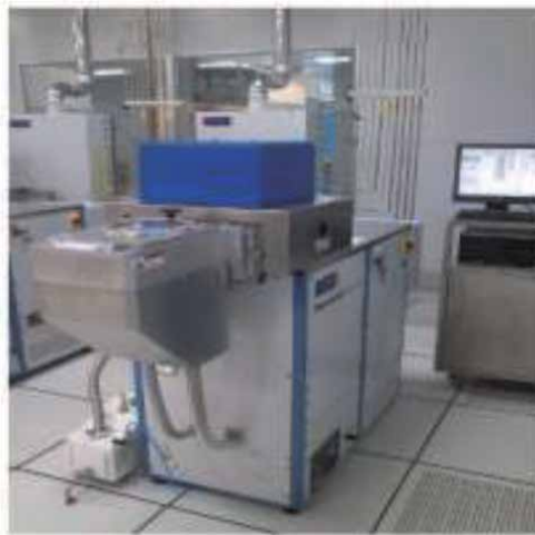
Figure 7. Oxford PECVD for Si 3 N 4 deposition at CeNSE.
