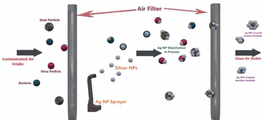
Figure 3. Anti-viral impact of silver nanoparticles on bioaerosols impregnated in the air filter. (Regenerated from reference [27]).
