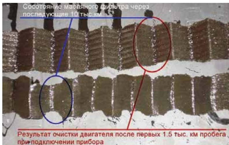
Fig. 16. Condition of the oil filters with the utilization of the ERF (above) and without it (below)
