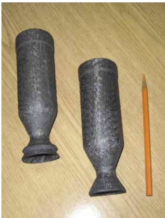
Fig. 7. Work material of ceramic combustion chamber.
