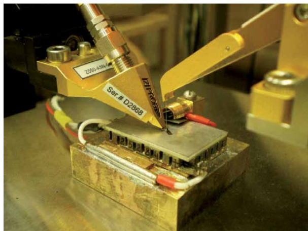
Figure 3. The workbench for VCSEL chip's study.
