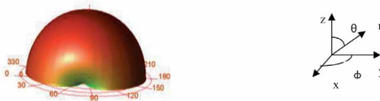
Figure 7. 3D radiation pattern for antenna with SRR.
