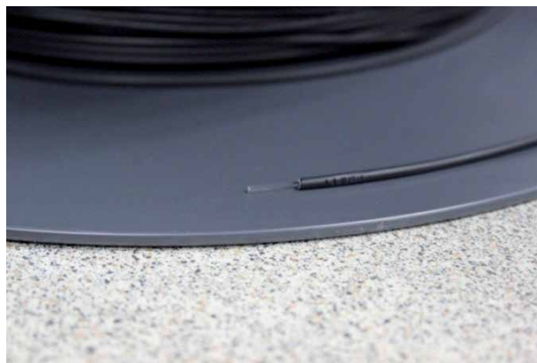
Figure 1. PMMA polymer optical fiber with diameter 1 mm.
