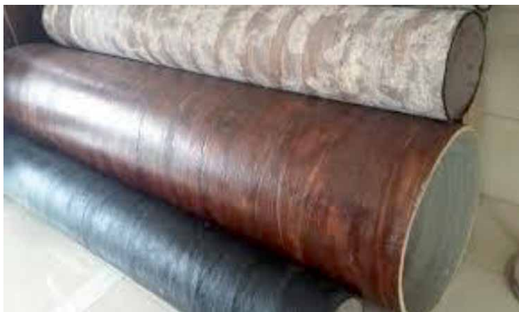
Figure 11. Bamboo winding composite pipes.
