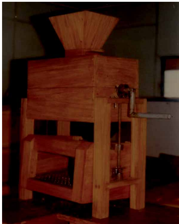
Figure 5. Modified wooden/metallic Sheller. Source: [20].
