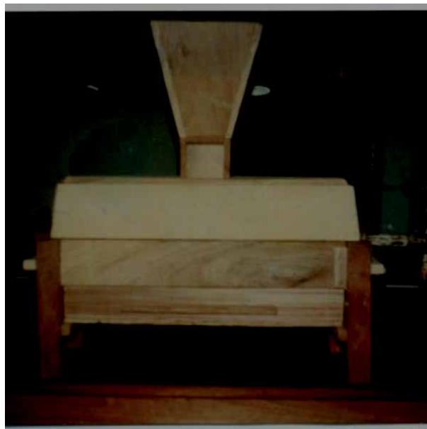
Figure 4. Wooden/metallic Sheller. Source: [19].
