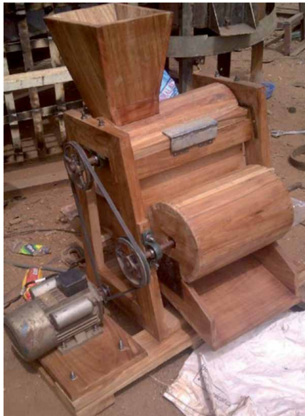
Figure 7. Wood-metal hybrid maize Sheller. Source: [27].
