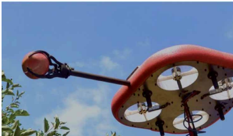
Figure 4. Flying autonomous robot in development for picking fruit, ( https://www.tevel-tech.com ).
