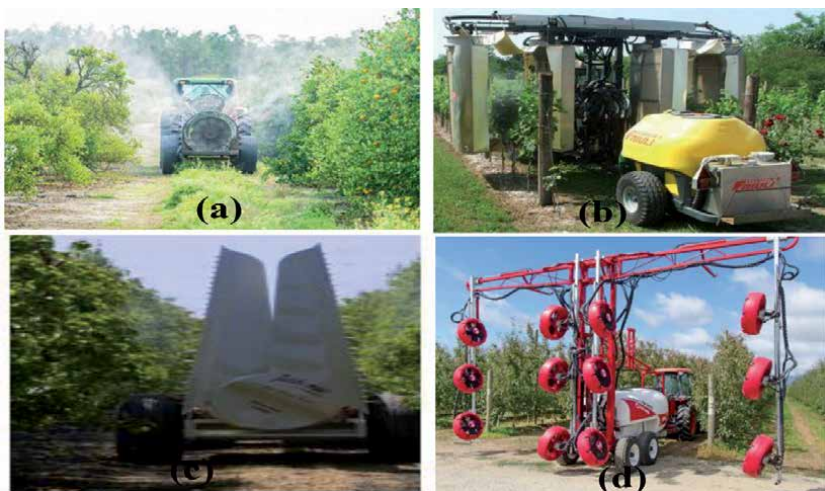
Figure 4. VAA orchard sprayer (a) tunnel sprayer (b) tower sprayer (c) multi channel air blast sprayer (d) [25].
