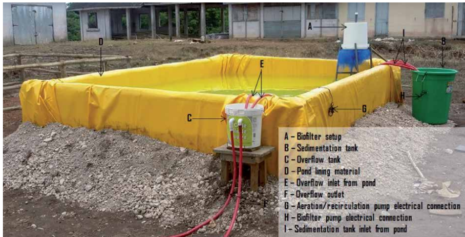
Figure 4. Parts of a typical recirculating aquaculture setup.
