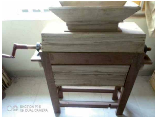
Figure 6. A completely wooden groundnut Sheller. Source: [21].
