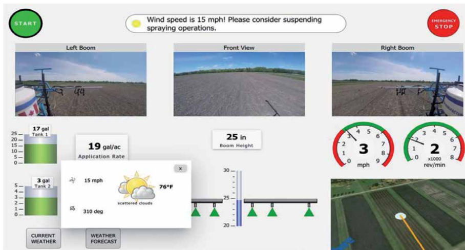
Figure 14. The automation interface designed for an autonomous plot-sized agricultural sprayer.
