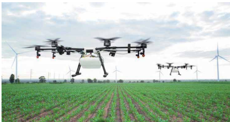
Figure 6. Group of drones capable of performing functions of high-definition maps of fields to create prescriptive-defined application of sprays, fertilizer, pesticides, herbicides and seeding.
