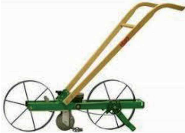
Figure 2. A planter in which wood is used for fabricating selected machine parts.
