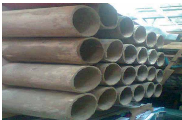
Figure 12. Cement-bonded composite pipes. Source: [35].
