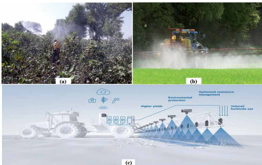
Figure 1. Cotton filed using Knapsack sprayer (a) wheat field using boom sprayer (b) schematic diagram of smart sprayer (c).
