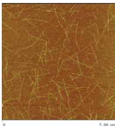
Fig. 7. Atomic force microscope image of synthesized imogolite.
