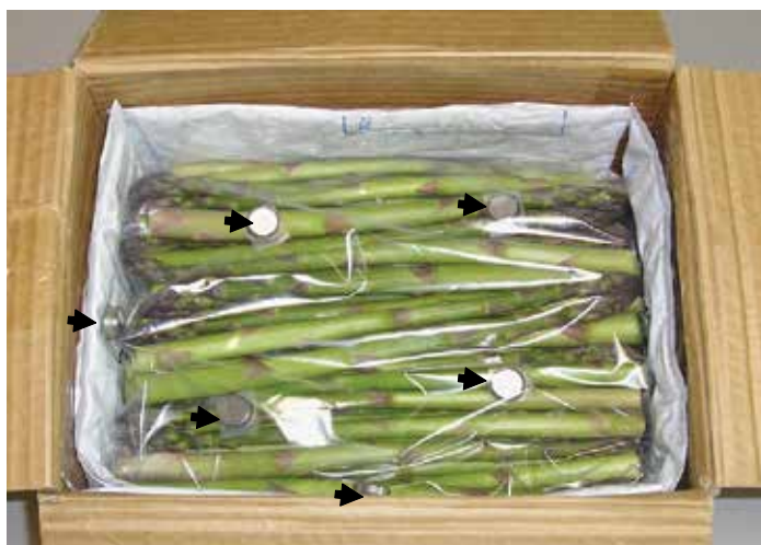
Fig. 6. Paperboard package with bubble wrap bag liners containing 400 g NCS-300PCM composite with RT6, and 2 kg of asparagus sealed in a polythene bag. The positions of the Dallas Semiconductor I-buttons used to measure the temperature / time profiles are shown by the arrows.
