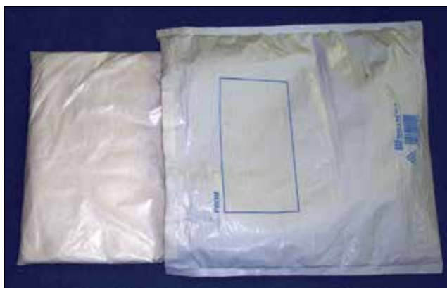
Fig. 3. The polythene bag containing a sample of NCS-PCM (left) being inserted into a bubblewrap bag (right).
