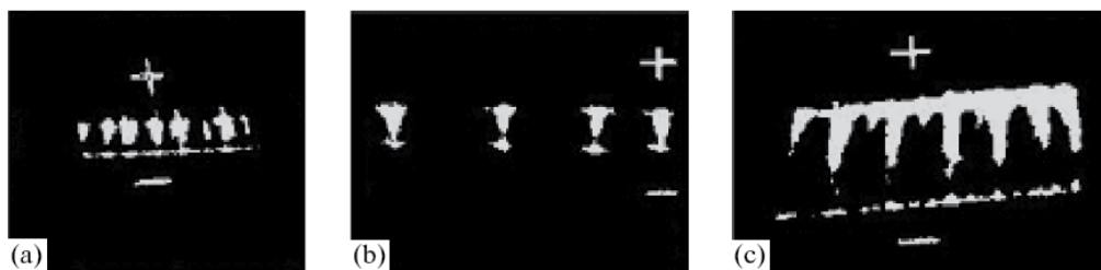
Fig. 26. Optical image of the development of microdischarges in the air medium between the dielectric (polytetrafluoroethylene with a thickness d = 2 \text{ mm} ) and the surface of the polymer solution. (a) d = 4 \text{ mm} , (b) d = 6 \text{ mm} , and (c) d = 10 \text{ mm} ; U = 35 \times 10^3 \text{ V} .
