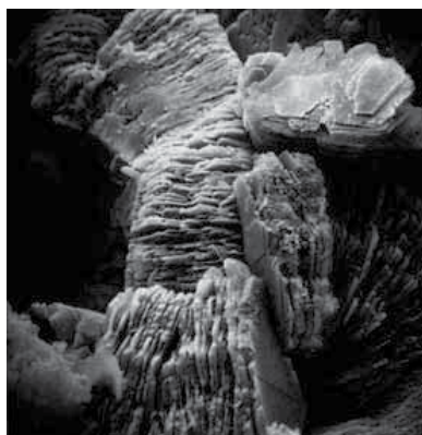
Fig. 3. Layers of naturally occurring phyllosilicate clay as seen under SEM.
