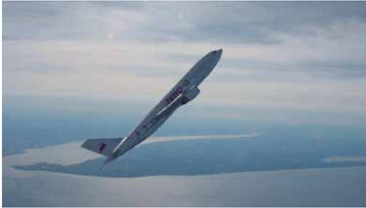
Figure 12. The Airbus A310 ZERO-G during the pull-up phase (Photo: Eric Magnan/Airborne Films).
