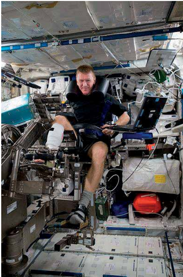
Figure 8. British ESA astronaut Tim Peake operates the muscle atrophy research and exercise system (MARES) equipment inside the Columbus module. MARES is an ESA facility used for research on musculoskeletal, biomechanical and neuromuscular human physiology to better understand the effects of microgravity on the muscular system (photo credit: NASA/ESA).
