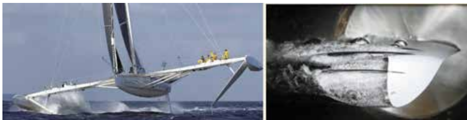
Figure 2. Left: the Hydroptère sailing boat (courtesy A. Thébaut) and right: evidence of cavitation on a model of the Hydroptère lifting foil.
