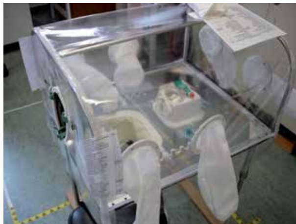
Figure 9. Hood system designed to avoid any possible blood contamination of the A300 cabin during the experiment.
