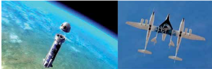
Figure 12. Two suborbital facilities in development: (left) the New Shepard capsule with a reusable rocket (credit: Blue origin) and (right) the WhiteKnightTwo airplane carrying the SpaceShipTwo spaceplane (photo credit: Virgin galactic).
