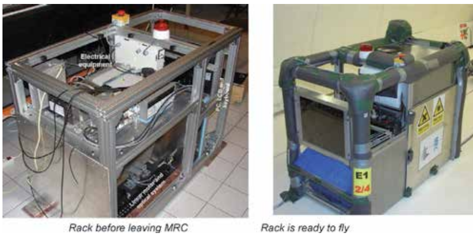
Figure 3. Rack designed for the TEVICON-1 parabolic flight experiment in 2007.
