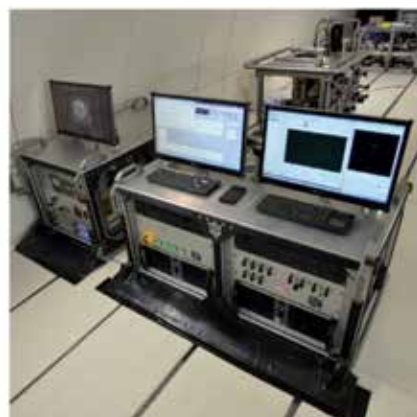
Figure 10. TEMPUS facility for parabolic flight. The authors share the experience of more than 3000 parabolas both in the NASA KC-135 and in the ESA-CNES-DLR Airbus A300s.
