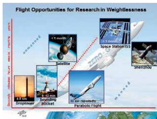
Figure 9. Reduced gravity platforms accessible to microgravity researchers (vertical axis, duration of microgravity; horizontal axis, quality of microgravity) (credit: DLR).
