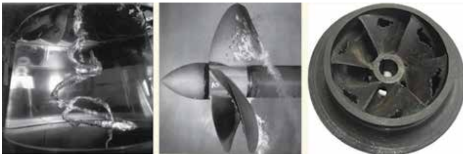
Figure 1. Left: cavitating vortex in a Francis turbine, operating at off-design conditions; middle: cavitation in a ship propeller (courtesy Franc et al. [4]); right: pump impeller heavily eroded by cavitation.
