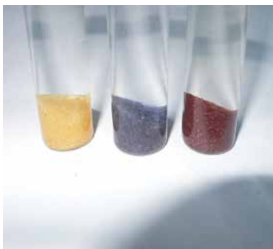
Fig. 1. Composite materials KU-2-Zn-m (pale yellow), KU-2-Ni-m (violet and turquoise disseminations) and KU-2-Cu-m (brown with metal lustre)
