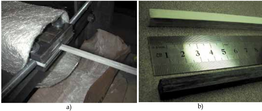
Fig. 12. a) Pultrusion die during manufacturing of Wo-CBPCs reinforced with glass fibers, b) pultruded bars of Wo-CBPCs reinforced with glass fibers (white) and with carbon fibers (black)
