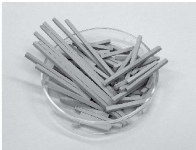
Fig. 9. General view of granulated Al 2 O 3 /Al composites prepared from powdered TCA and PA-4 used as supports for dehydrogenation catalysts.
