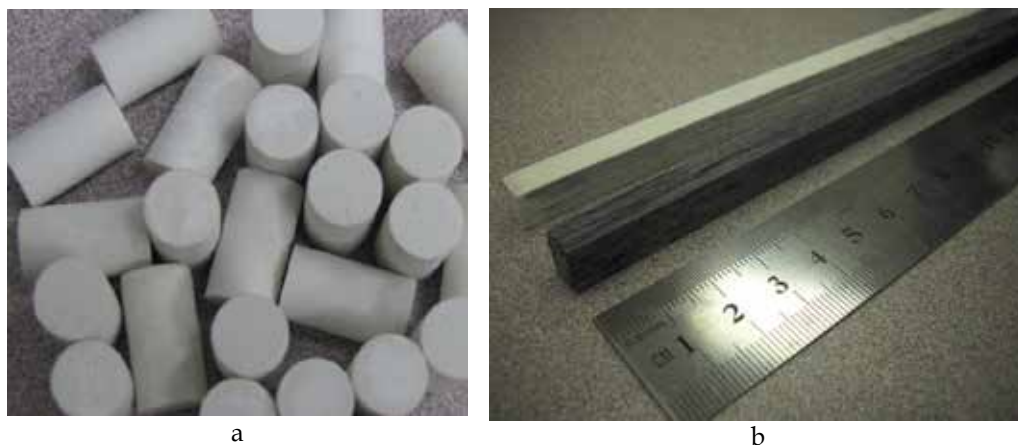
Fig. 1. Wollastonite-based CBPCs, a) compression samples, b) pultruded bars of CBPCs reinforced with glass fibers (white) and with carbon fibers (black).
