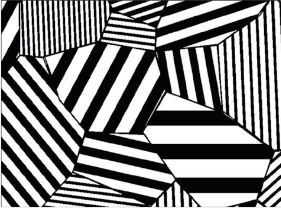
Fig. 1. Schematics of polycrystals with anisotropic grains (from Schulgasser 1977)
