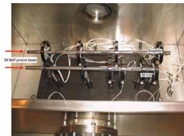
Fig. 4. C/C composite and ATJ graphite target shock test arrangement for the BNL AGS proton beam tests
