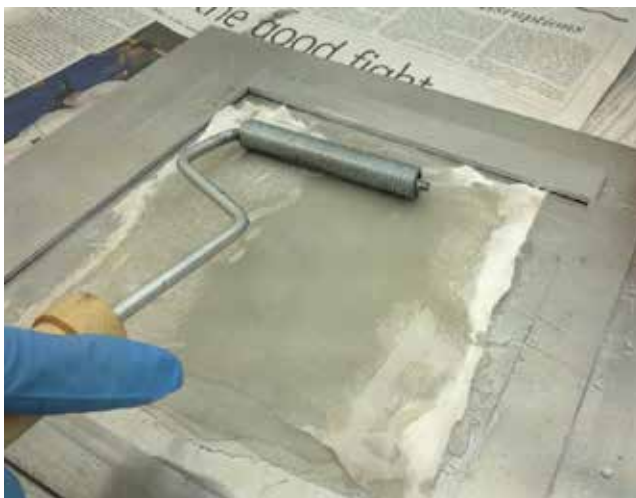
Fig. 4. Wet layup of silk fabric
