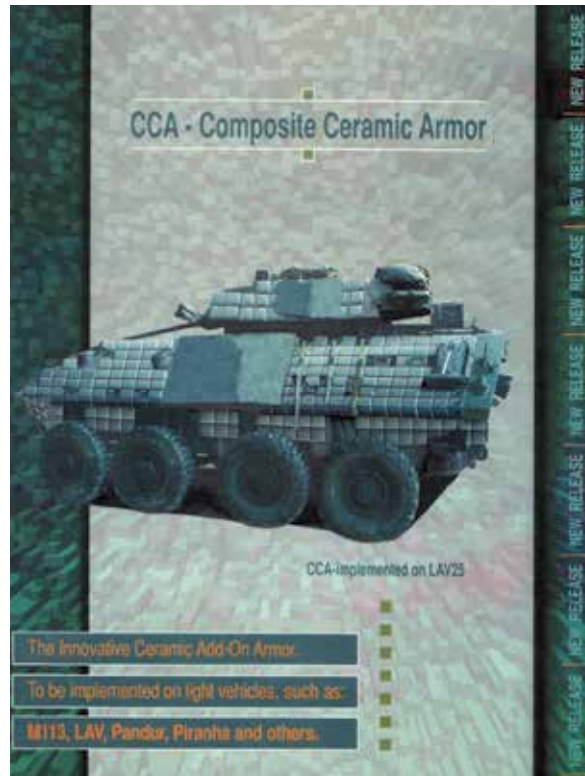
Fig. 4. Composite boroncarbide ceramic plates on armored vehicle ( Company Rafael - Israel)
