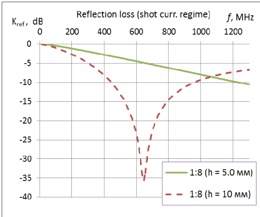
Fig. 6. The reflection coefficient of the composite materials on the basis of Ni-Zn ferrite. (Two thicknesses of the samples).
