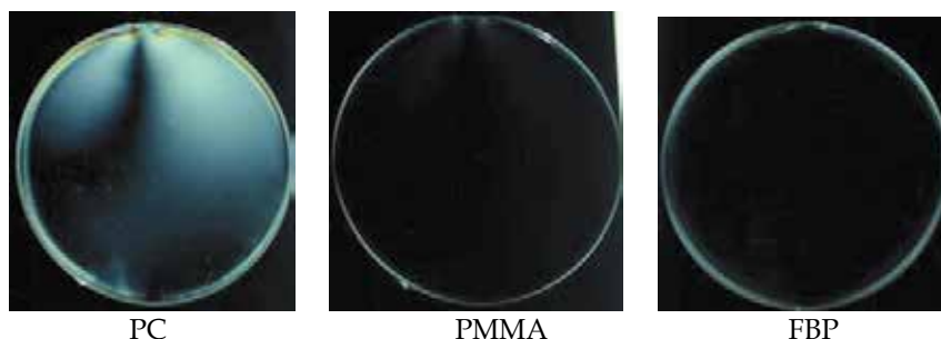
Fig. 3.2.2.1. Birefringence property of optical polymers.
