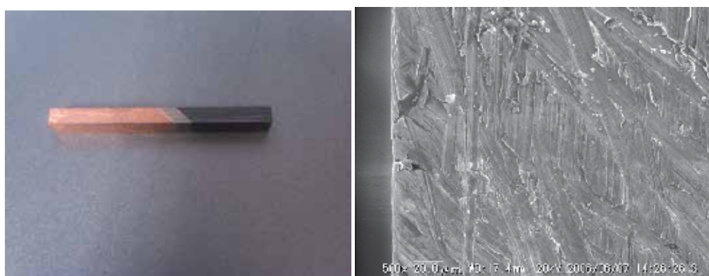
Fig. 22. Graphite-titanium-copper composite sample (left) used for the BNL irradiation studies and SEM image of the copper-titanium interface prior to irradiation
