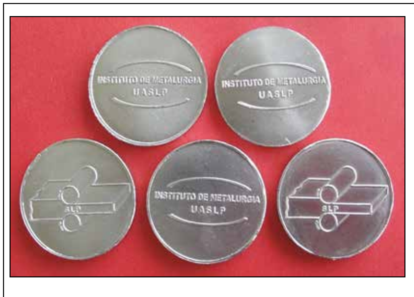
Fig. 14. Medals elaborated with aluminum clad zinalco.
