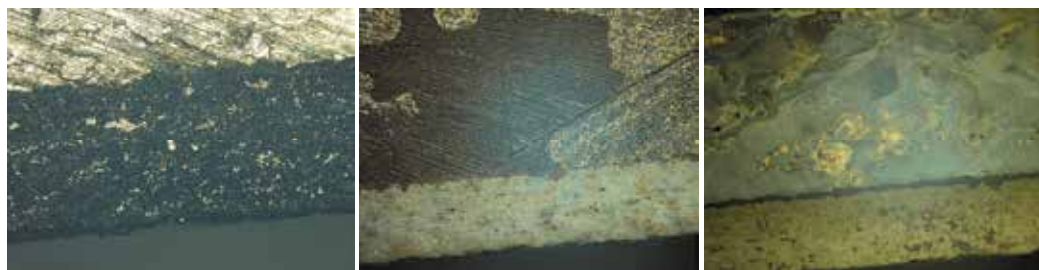
Fig. 25. Effect of temperature on the interface of nano-structured alumina coating on Ti-6Al-4V substrate from room temperature (left), to 900°C (middle) and 1200°C (right)
