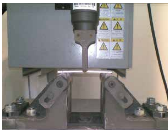
Fig. 10. Three point bending test setup
