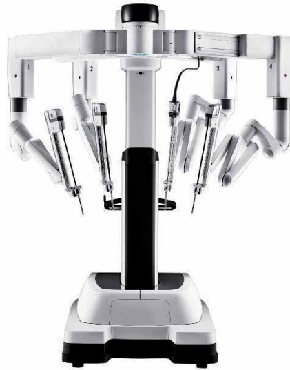
Figure 1. Da Vinci XI patient cart with four robotic arms. Image courtesy of © [2020] Intuitive Surgical, Inc.
