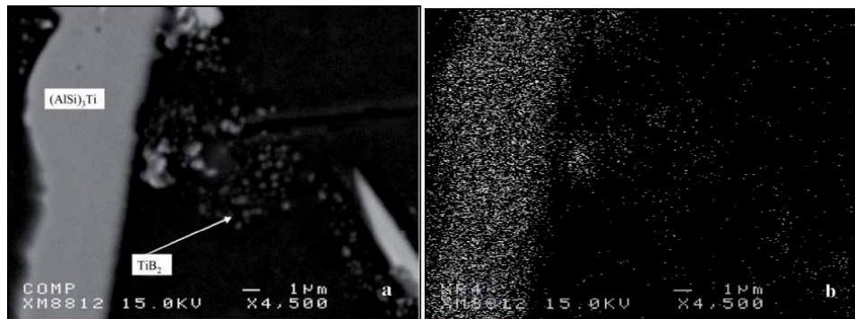
Figure 5. Decomposition of the added Al-5%Ti-1%B master alloy: (a) backscattered electron image, (b) X-ray image of Ti distribution.
