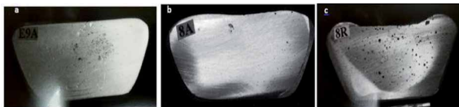
Figure 1. RPT test taken from: (a) as received alloy, (b) after degassing, (c) 0.25 ml/100 g H_2 .
