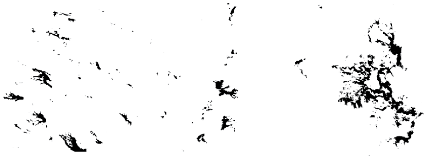
Figure 14. Morphologies of linear (left) and feathery (right) shrinkage porosity.
