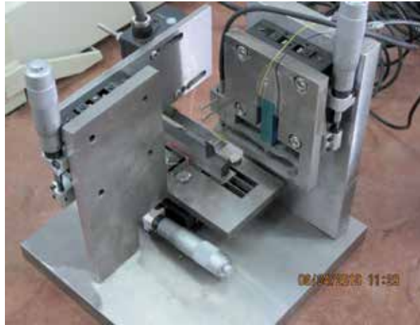
Fig. 21. Prototype of designed indentation device
