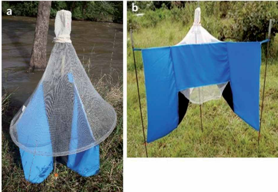
Figure 2. Trap types a) vavoua trap, b) nzi trap (photos by Sevidzem SL).
