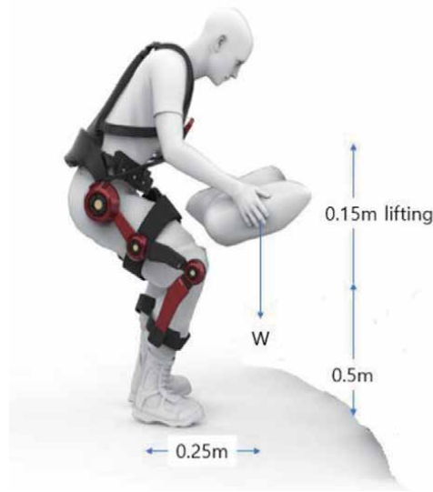
Figure 4. Weight lifting motion with waist and knee exoskeleton robots.
