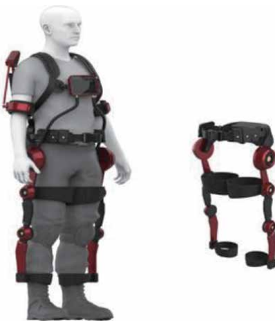
Figure 1. The concept design of modular exoskeleton robot.
