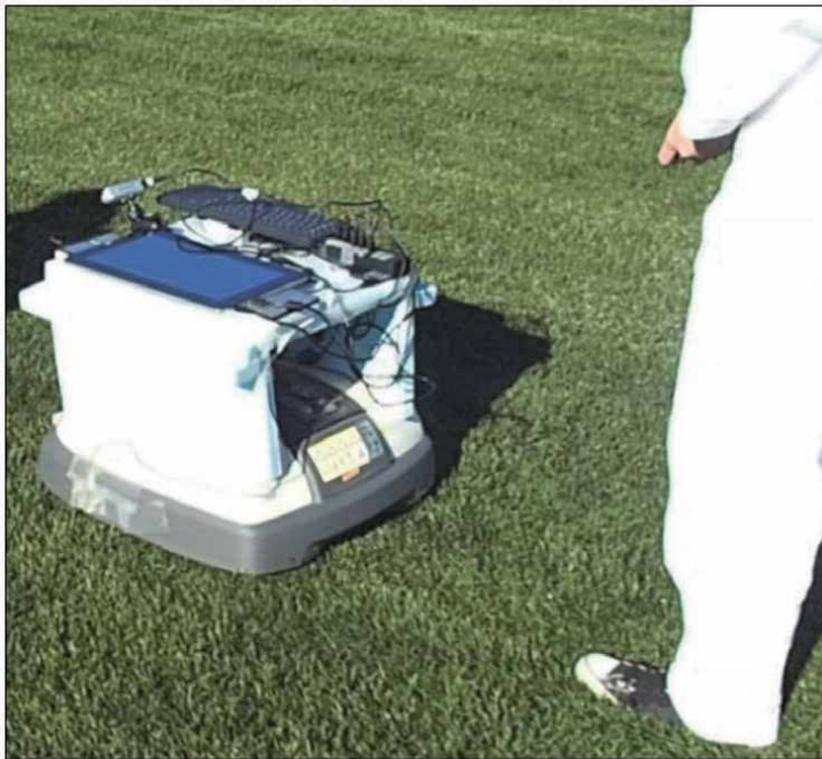
Figure 7. Remote-controlled driving of Robo-mower.
