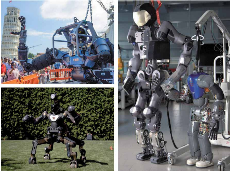
Figure 10. XBot framework usage examples: WALK-MAN robot in Pisa (top left), CENTAURO robot untethered and outdoor (bottom left), and the COMAN and its scaled-up version COMAN+ humanoid robots shaking hands (right).
