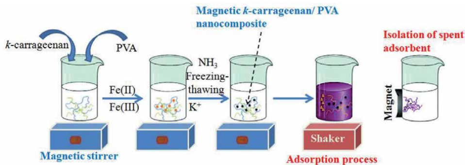
Figure 7. Fabrication of magnetic kC/PVA nanocomposite as an adsorbent for cationic dye removal in aqueous solution.
