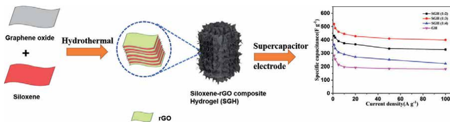
Figure 4. Synthesis of siloxene-reduced graphene oxide hydrogel and its specific capacitance plot [26].
