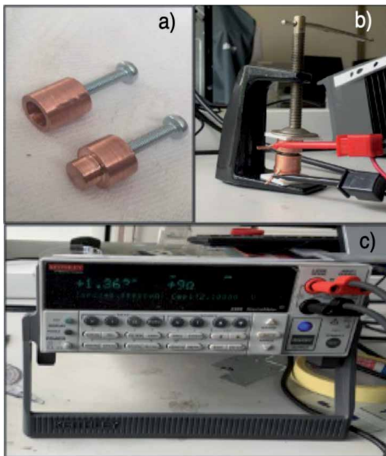
Figure 6. Electrical resistivity measurement system: (a) copper cylindrical container and a copper cap. (b) Electrical resistivity measurement set-up (joiner's clamp and copper container). (c) Keithley 2400 Sourcemeter.
