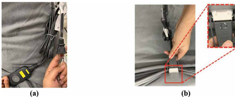
Figure 6. Resistive heating blanket: (a) electronic control module with wiring for power supply; (b) connection between electronic module and the blanket (identified with the red box). The rigid connector is sewn to the blanket with a single row of stitches (shown in the inset).
