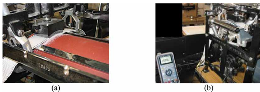
Figure 4. Abrasion testing on a white webbing with conductive yarns (a). A multimeter measured the change in resistance after successive series of abrasion cycles (b).
