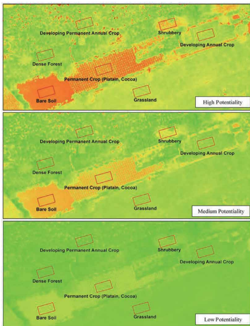
Figure 3. Vegetation indexes with RGB data, classified according to their potential to discriminate different types of land cover.
