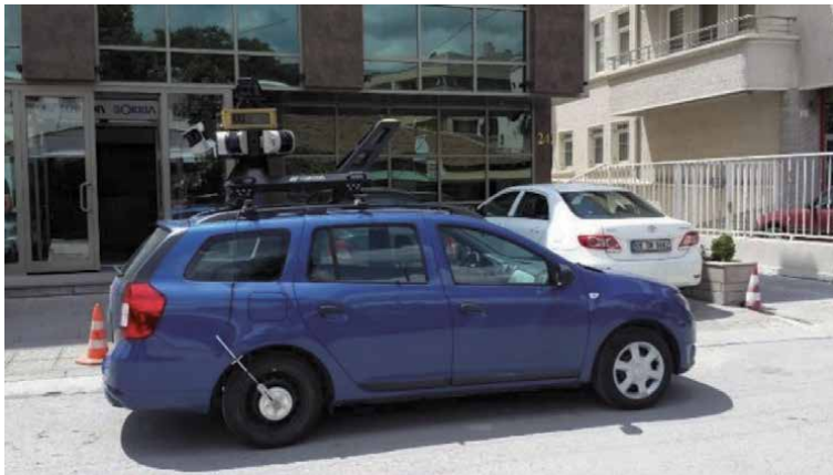
Figure 16. The vehicle of application which was used to obtain point cloud data.
