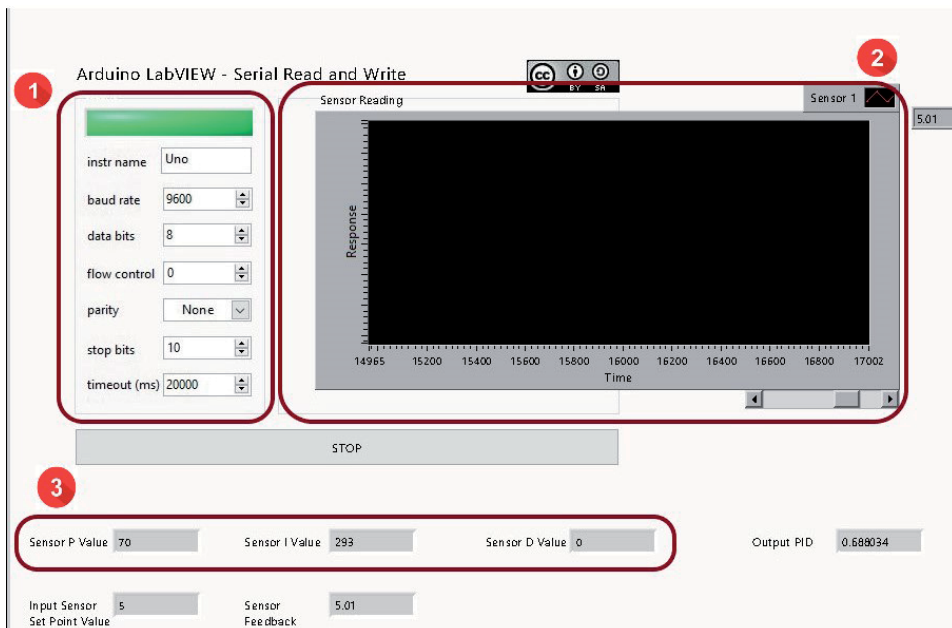
Figure 8. VIs from the front panel of the PID control and monitoring system (1) Arduino-LABVIEW serial read and write (2) waveform chart (3) PID setting parameters.
