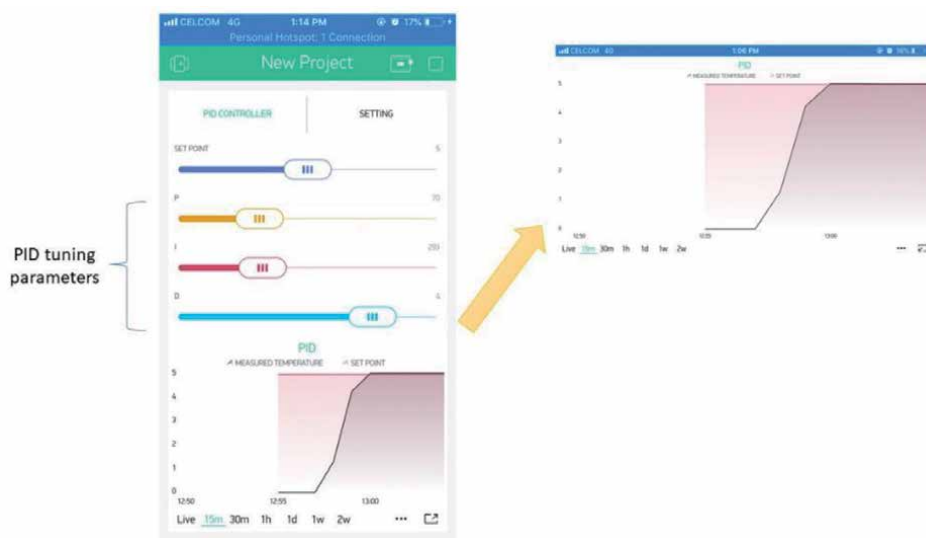
Figure 9. Blynk interface with widgets configured for remote monitoring.
