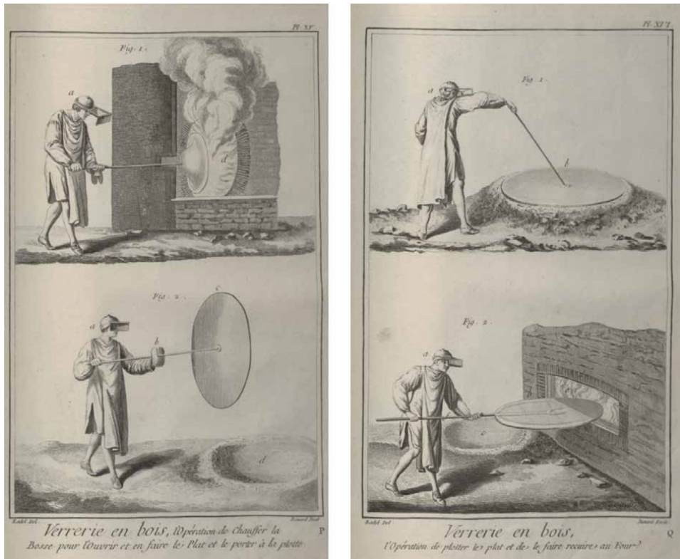
Figure 7. Robert Bénard (French artist, 1734–1777). Crown or window glass making engraving plates. Plates XV & XVI from [75]. The description (in French) of particular craft operations is also available online at [75].
