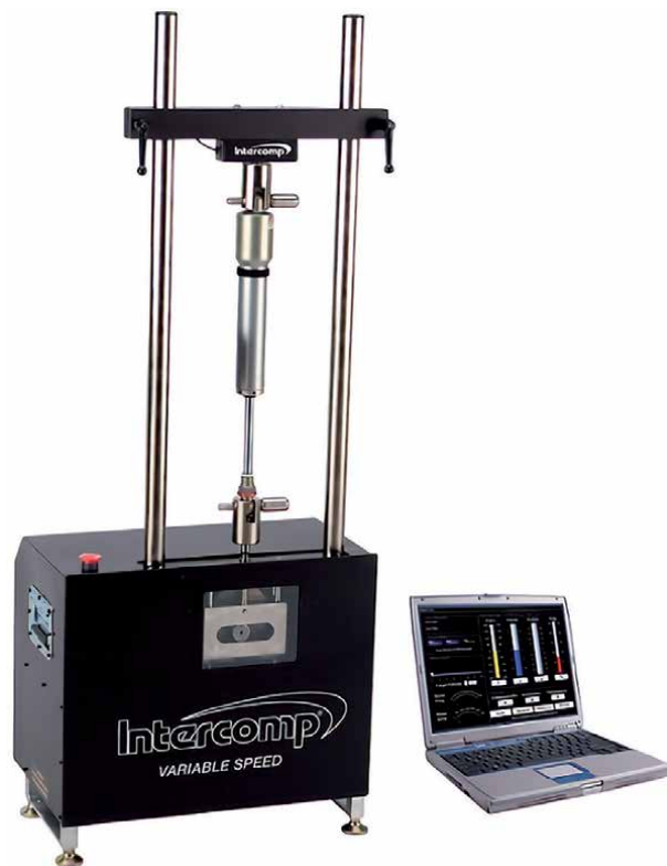
Figure 2. Intercomp 3HP shock dyno 1.0–55 in/s ($8895.00).
