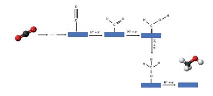
Figure 4. Schematic of possible pathways for methanol production.
