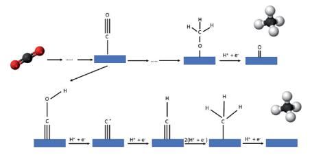
Figure 3. Schematic of possible pathways for methane production.
