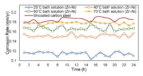
Figure 8. LPR corrosion rate measurements taken for Zn-Ni alloy coatings vs. uncoated carbon steel for hourly for 24 h.
