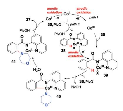
**Figure 17.** A plausible mechanism for C-N bond formation by Co-catalysis.
