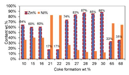
**Figure 10.** EDX results of C content (wt.%) in terms of Zn-Ni compositions after 48 h of electrochemical  $CO_2RR$ .
