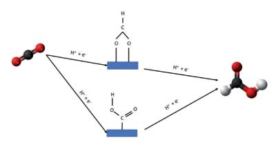
Figure 2. Schematic of possible pathways for formic acid production.
