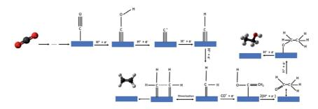
Figure 5. Schematic of possible pathways for ethylene and ethanol CO production.
