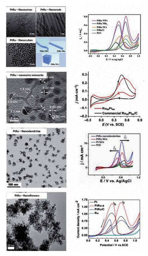
Figure 6. TEM images and CV curves of the various morphologies of PtRu [87–90].
