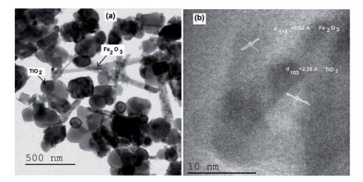
**Figure 1.** HRTEM image of: (a)  $Fe_2O_3/TiO_2$ , (b) HRTEM lattice fringe image of:  $Fe_2O_3/TiO_2$ .
