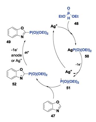
**Figure 21.** *A plausible mechanism for C-P bond formation by Ag-Catalysis.*
