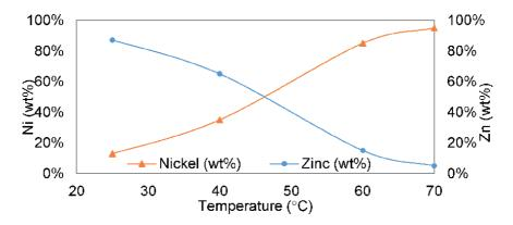
**Figure 7.** EDX analysis results in terms of Zn and Ni contents (wt%) vs. bath solution temperature (°C).
