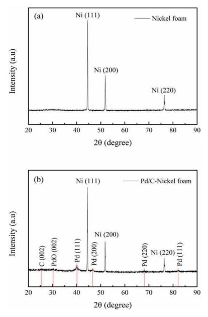
**Figure 2.** *XRD pattern of (a) the clean Ni foam and (b) the Pd/C-Ni foam electrode.*
