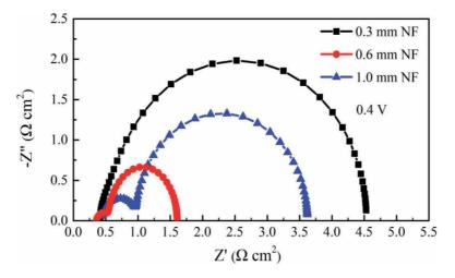
**Figure 5.** EIS comparison of ADEFC with different thickness of Ni foam electrodes at 0.4 V.
