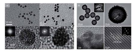
Figure 7. TEM and HR-TEM images of core-shell (a) and Pt@mPtRu Yolk – Shell (b) nanostructures [93, 94].
