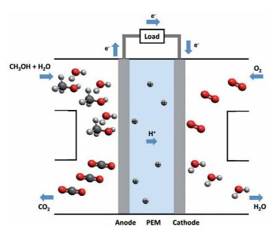
**Figure 1.** *Structure and operating principle of DMFC.*
