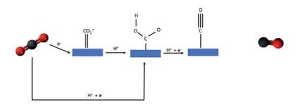
Figure 1. Schematic of possible pathways for CO production.
