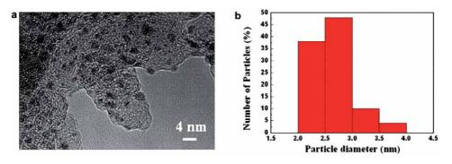
**Figure 4.** *A TEM image (a) and particle size distribution (b) of PtRuFe/C (2:1:1) catalyst [43].*
