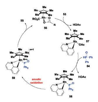
Figure 23. Plausible mechanism for Rh(III)- catalyzed electrochemical phosphorylation of aryl substrates.
