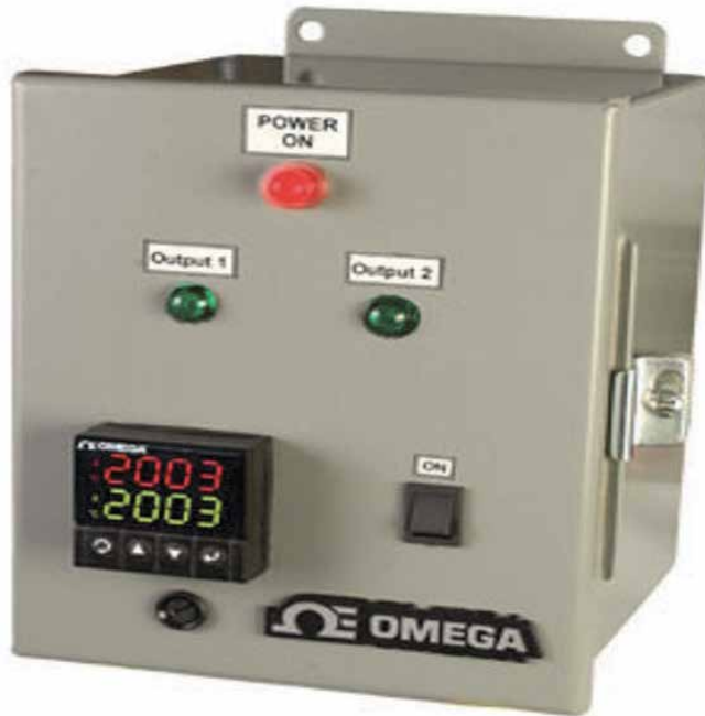
Figure 2. Temperature control box for storing the prepared blend in various temperatures.
