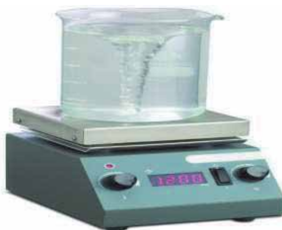
Figure 1. Magnetic stirrer used for the blend preparation.
