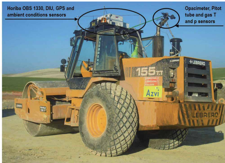
Figure 7. View of the experimental installation located on the construction machine.
