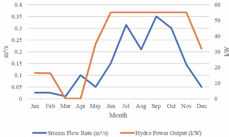
Figure 15. Stream flow rate and power output of the micro-hydro (adapted from [35]).
