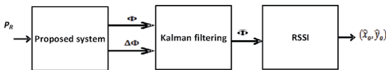
Figure 5. The block diagram of the proposed system with KF.
