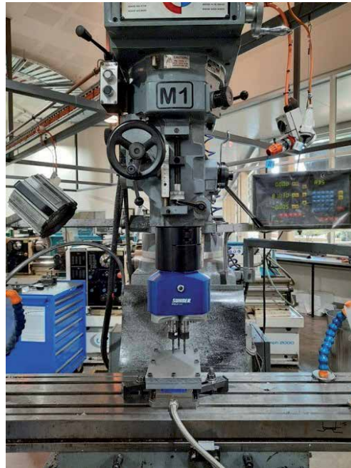
Figure 5. The 3-spindle Suhner multi-spindle drill head mounted on conventional milling machine (Courtesy: Edith Cowan University, Australia).
