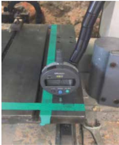
Figure 4. Verification of the surface flatness of the table.
