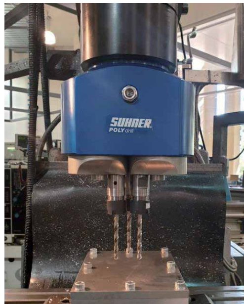
Figure 2. A poly-drill head with three adjustable spindles mounted on conventional milling machine.
