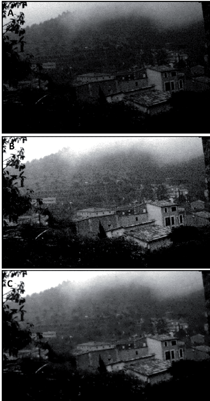
Figure 3. Performance of the NV algorithm using a dim natural image as input. (A) Noisy image of a village on Mallorca (printed with permission from Buades; see Buades et al. [6]). (B) Noise was amplified after histogram stretching. (C) The output of the NV algorithm yielded a reduced amount of noise (PSNR = 35.3 dB) and shows a higher quality regarding image details and contrast.
