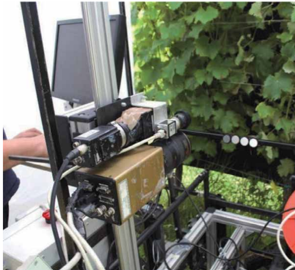
Figure 10. Camera setup for the agricultural robot [8].
