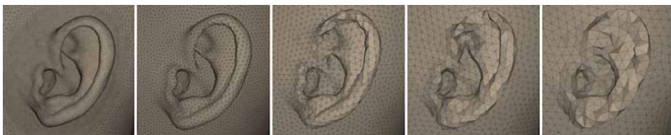
Figure 8. Pinna meshes represented by various AELs [90]. From left to right: AEL of 1 mm, 2 mm, 3 mm, 4 mm and 5 mm. Note how the representations of the helix and fossa triangularis degrade with increasing AEL.
