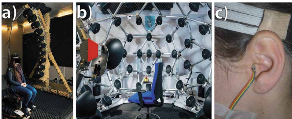
Figure 6. (a) Example of an HRTF measurement setup with mechanical rotation required. Listener sits on a chair (mounted on a turntable) surrounded by a loudspeaker arc (22 loudspeakers ranging from -30 to 210^\circ in 5^\circ -steps). A head-tracker mounted on the head of the listener tracks head movements, triggering the need for measurement repetition in case of too large movements. (b) Example of more recent HRTF setups. 91 loudspeakers are mounted in a near-complete spherical array reducing the total measurement duration. (c) Example for a microphone placement in an HRTF measurement. Note the closed ear canal and the head-tracker sensor.
