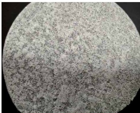
Figure 8. Picture of porous structures obtained by the porophor agent washout method.
