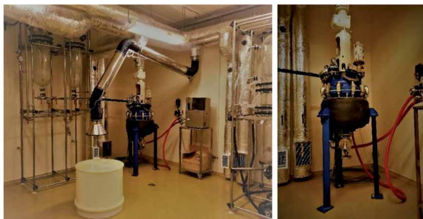
Figure 5. Set for the synthesis of butyryl-acetyl chitin co-polyester on an industrial scale.
