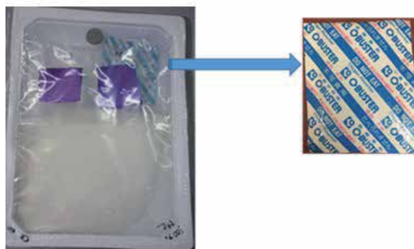
Figure 4. A schematic illustration of smart (active + intelligent) packaging system for mozzarella cheese package with oxygen indicator (shown in pink color) and oxygen scavenger (O-buster® oxygen scavenger) (Source: [15]).
