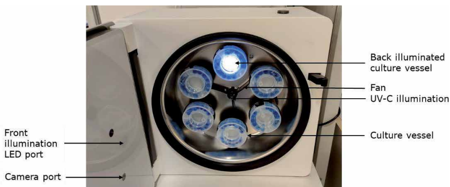
Figure 7. A clinostat incubator, containing 6 culture vessels (one back illuminated).
