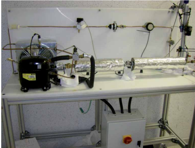
Figure 10. VC system to test nano-lubricant effects on COP.
