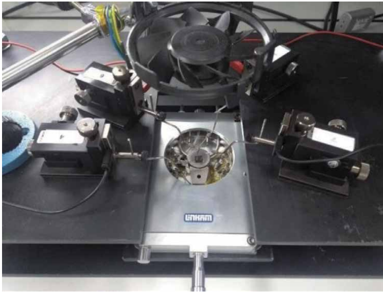
Figure 6. Experimental setup used for the thermoelectrical characterization of \mu TEG devices under a forced convection regime induced by a CPU fan located on the top. The device is mounted on the thermal chuck of a Linkam station.
