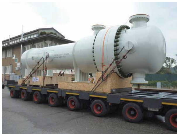
Figure 20. EMbaffle® overhead gas cooler.
