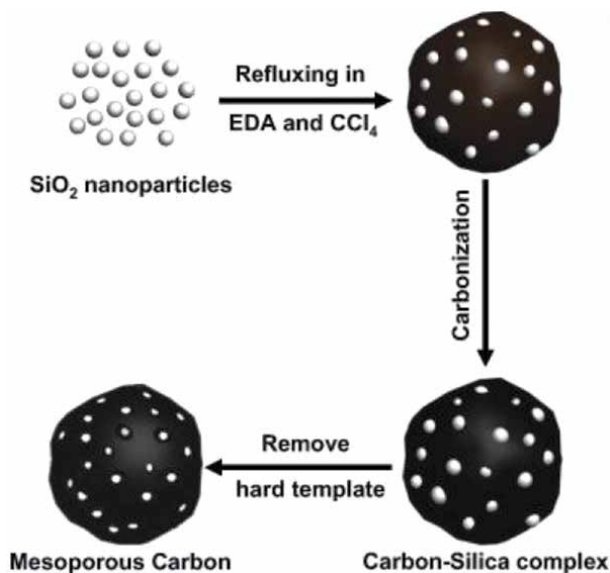
Figure 4. Preparation of mesoporous carbon using silica porous matrix [53].
