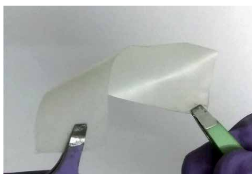
Figure 5. Flexibility and mechanical stability of IL based gel polymer electrolyte.
