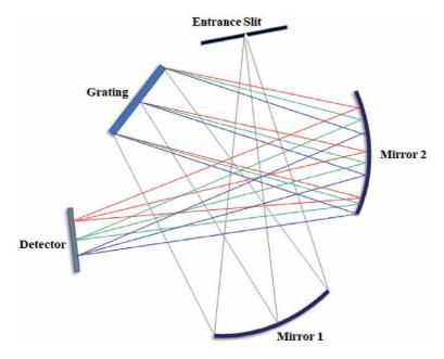
Figure 1. Dispersive spectrometer based on the Czerny-Turner design [16].
