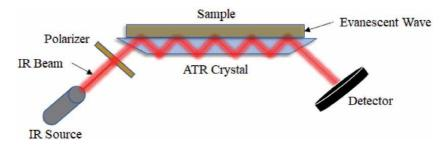
**Figure 7.** Diagram illustrating the ATR concept [28].
