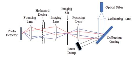
Figure 4. Basic design layout for a Hadamard spectrometer [23].
