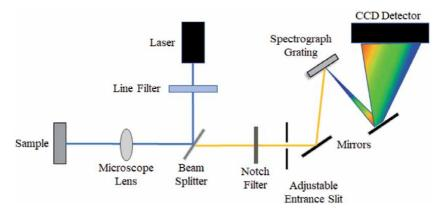
Figure 8. Basic diagram of a Raman spectrometer [31].
