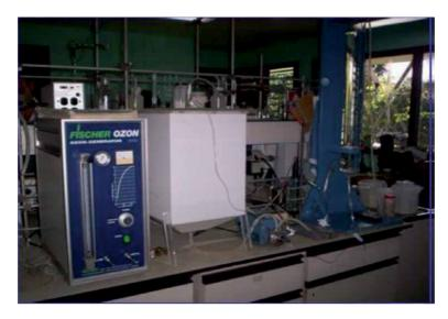
**Figure 8.** *Equipment used for the ozonation of water.*
