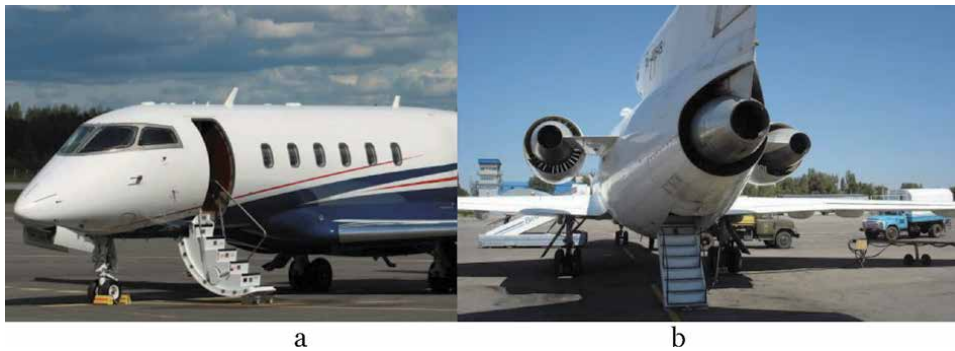
Figure 32. The door stairs at passenger airplanes: (a) side location for Bombardier Challenger 300; (b) rear location for Yakovlev Yak-42.
