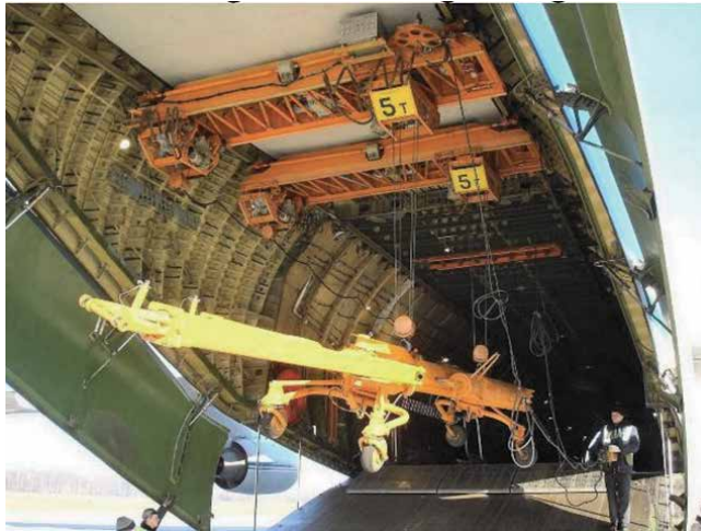
Figure 25. Cargo compartment with the built-in hoist of the cargo aircraft Antonov An-124.
