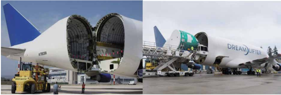
Figure 28. Rear cargo door of “Dreamlifter” B747.
