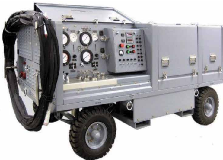
Figure 8. Special equipment for hydraulic system checking.
