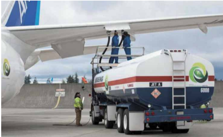
Figure 21. Airplane fueling from the service car—non-rational.
