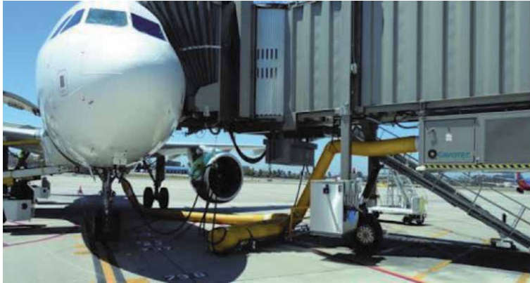
Figure 12. Some airports have passenger boarding bridges that supply air-conditioning, ground power, potable water, etc.
