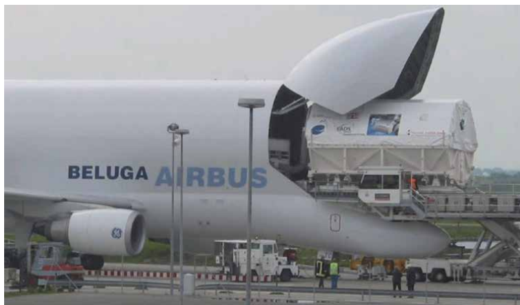
Figure 29. Loading cargo into Airbus beluga cargo plane from nose cargo door.
