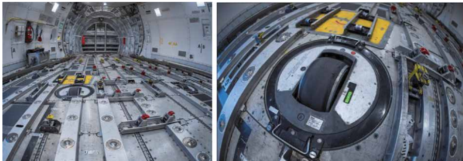
Figure 24. Floor of the airplane B747 cargo compartment with the devices for moving and fastening of cargo.
