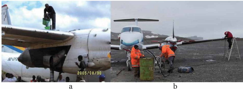
Figure 23. Handle refueling aircraft: (a) Antonov An-26 in Africa; (b) Beechcraft 300 at the Antarctic Air Base Pot. E. Frei M.
