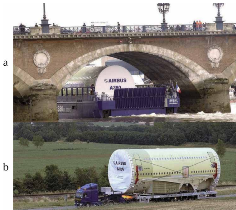
Figure 42. Transportation of Airbus A380 section: (a) fuselage by river ship; (b) fuselage by road.
