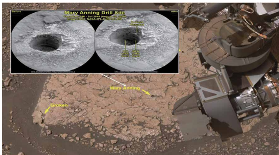
Figure 47. The Mary Anning drill site (Glen Torridon clay unit) where the first TMAH derivatization was performed on September 2020.
