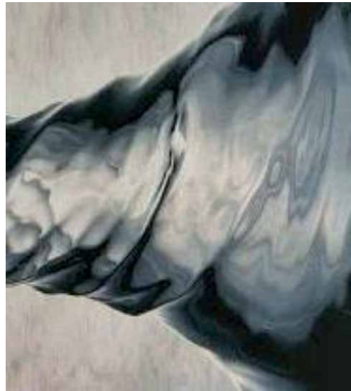
Figure 5. View of a corkscrew vortex flow in fluid dynamics. Its geometry is equivalent to that of a vortex flow in the Venus wake with its width and position varying during the solar cycle. Near minimum solar cycle conditions the vortex is located closer to Venus (right side) and there are indications that its width becomes smaller with increasing distance downstream from the planet. Such is the case for orbits within the left circle of Figure 4 and that were conducted before the solar cycle minimum at 2009–2010 thus implying that it becomes thinner when it is detected further downstream along the wake.
